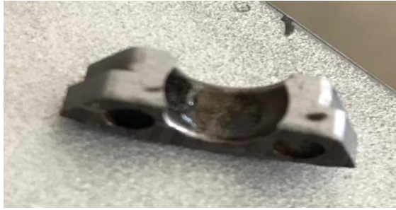
Figure 6.20 The final shape of the secondary middle part focusing on the rounded surface.
