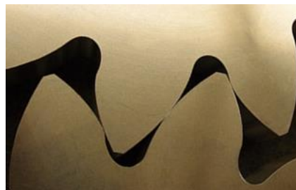
Figure 1.1 Asymmetric involute gear tooth profile
