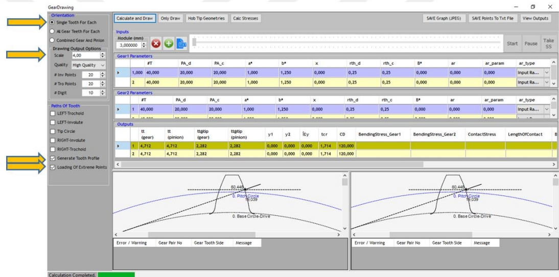
Figure 3.35 Loading gear teeth at highest point of single tooth contact (HPSTC)
