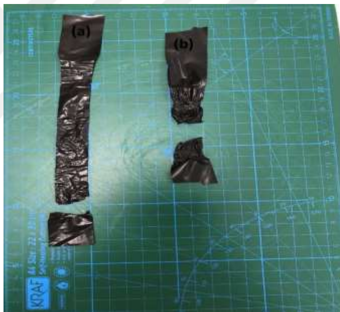
Figure 4.12 %90 F2-12 + %10 (LDPE/10 wt.% graphene) (a) Machine Direction Break Form (b) Transverse Direction Break Form
