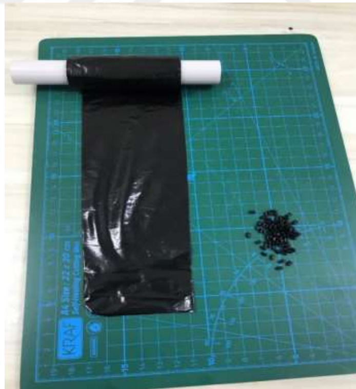
Figure 4.3 95% F2-12 + 5% Graphene (LDPE/5 wt.% graphene)
