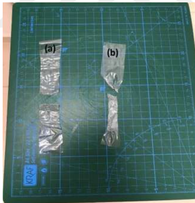
Figure 4.8 %90 F2-12 + %9.9 Calcite + %0.1 Graphene (LDPE/0.1 wt.% graphene) (a) Machine Direction Break Form (b) Transverse Direction Break Form
