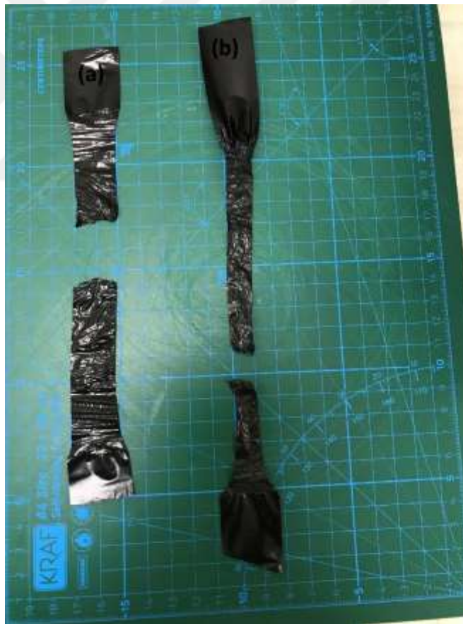
Figure 4.10 %95 F2-12 + %5 (LDPE/5 wt.% graphene) (a) Machine Direction Break Form (b) Transverse Direction Break Form Diagram
