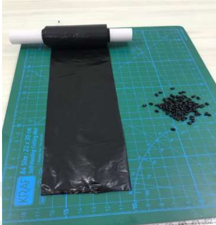
Figure 4.4 90% F2-12 + 10% Graphene (LDPE/10 wt.% graphene)
