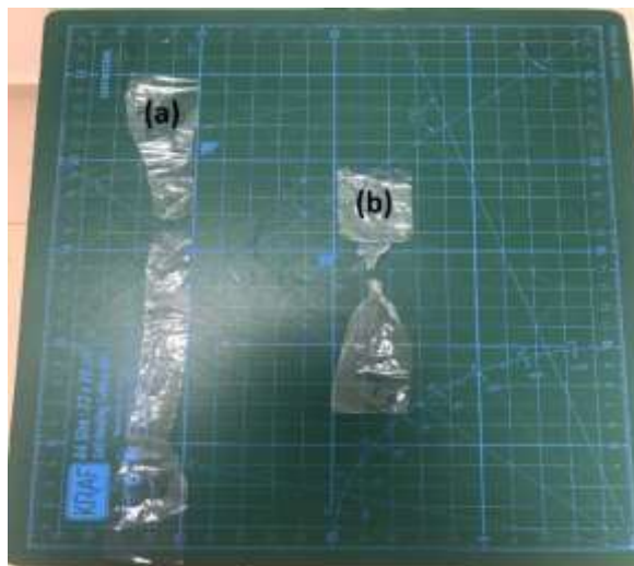
Figure 4.6 %100 F2-12 (pure LDPE film) (a) Machine Direction Break Form (b) Transverse Direction Break Form
