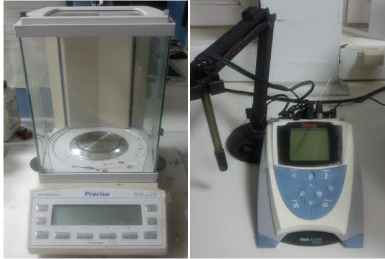
Şekil 3.2. A. PRECİCA XR 205SM-DR model hassa terazi ve B. ORİON STAR SERIES marka pH metre
