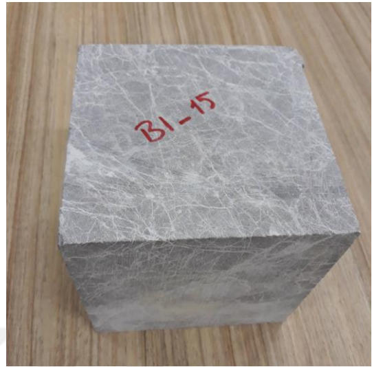
Figure 4.21. Post-thermal damage–B1-15 (at 500°C)
