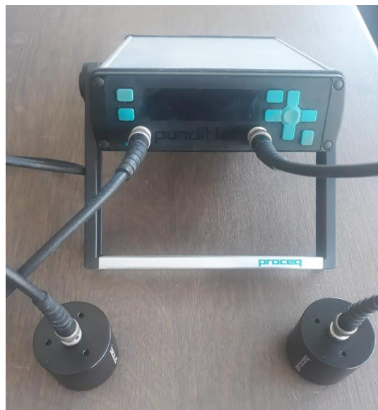
Figure 3.5. PROCEQ Ultrasonic Pulse Velocity Tester
