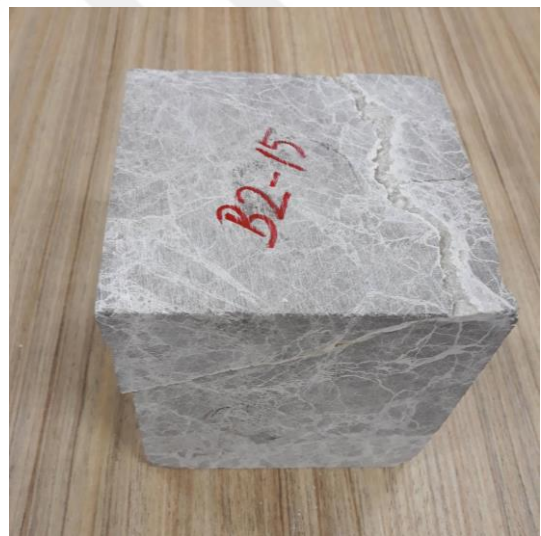
Figure 4.23. Post-thermal damage–B2-15 (at 500°C)
