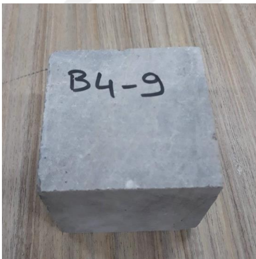
Figure 4.46. Pre-thermal damage–B4-9 (at 0°C)
