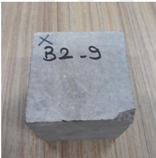
Figure 4.42. Pre-thermal damage-B2-9 (at 0°C)
