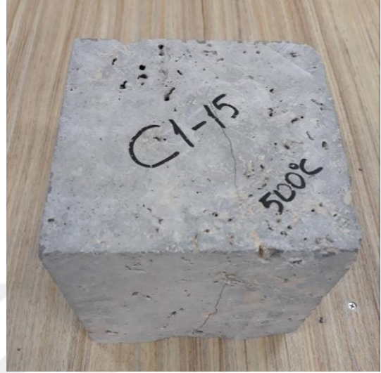
Figure 4.29. Post-thermal damage–C1-15 (at 500°C)
