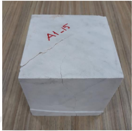
Figure 4.13. Post-thermal damage–A1-15 (at 500°C)
