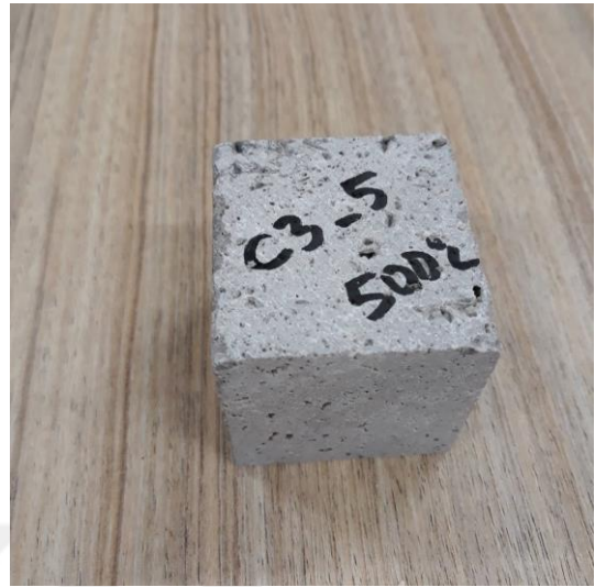
Figure 4.77. Post-thermal damage–C3-5 (at 500°C)
