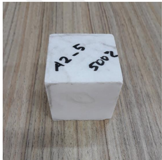
Figure 4.59. Post-thermal damage–A2-5 (at 500°C)
