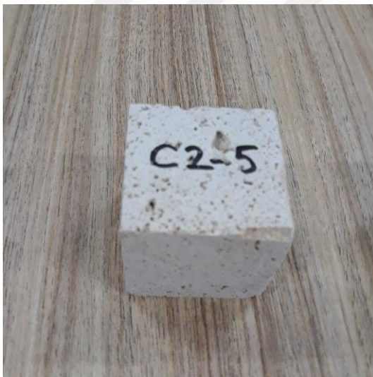
Figure 4.74. Pre-thermal damage-C2-5 (at 0°C)
