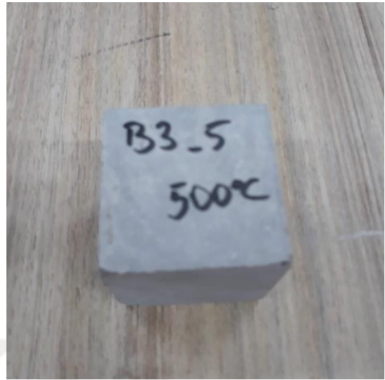
Figure 4.69. Post-thermal damage-B3-5 (at 500°C)
