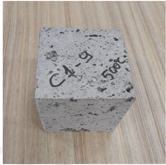
Figure 4.49. Post-thermal damage–C1-9 (at 500°C)
