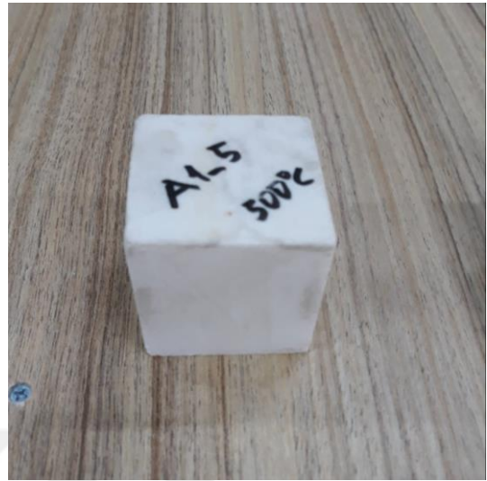
Figure 4.57. Post-thermal damage–A1-5 (at 500°C)
