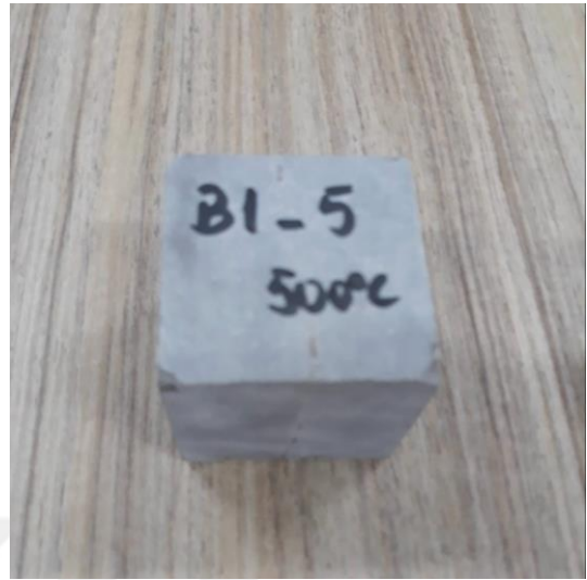
Figure 4.65. Post-thermal damage-B1-5 (at 500°C)
