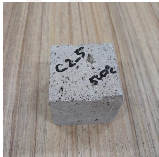
Figure 4.75. Post-thermal damage-C2-5 (at 500°C)
