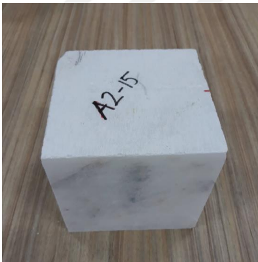
Figure 4.14. Pre-thermal damage–A2-15 (at 0°C)
