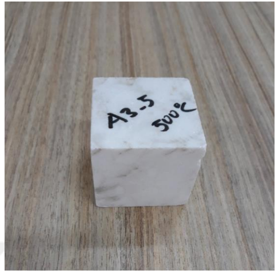
Figure 4.61. Post-thermal damage–A3-5 (at 500°C)
