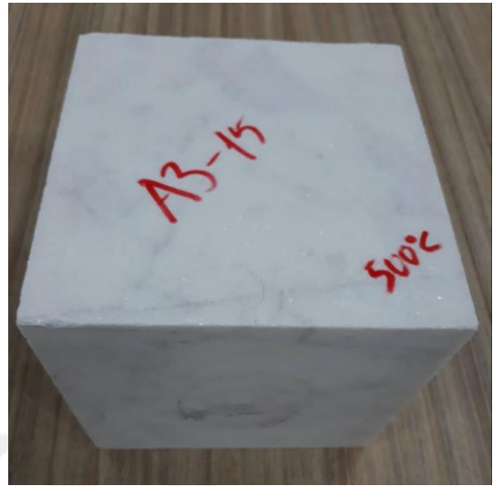
Figure 4.17. Post-thermal damage–A3-15 (at 500°C)
