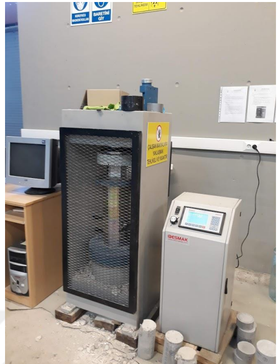
Figure 3.7. The Uniaxial Compressive Strength Testing Device
