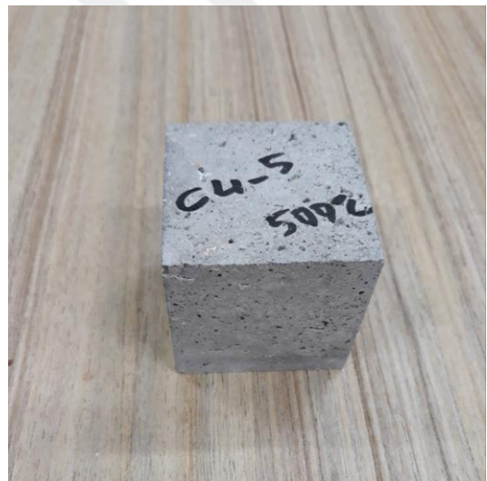
Figure 4.79. Post-thermal damage–C4-5 (at 500°C)
