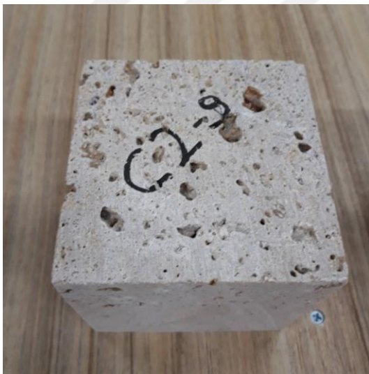
Figure 4.50. Pre-thermal damage–C2-9 (at 0°C)
