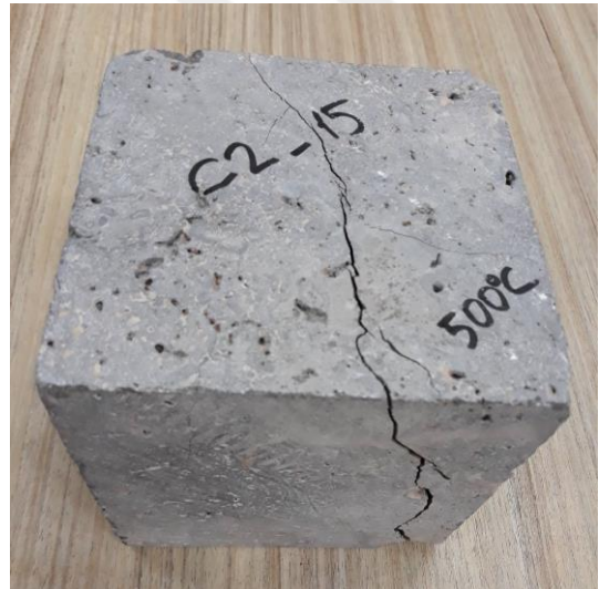
Figure 4.31. Post-thermal damage–C2-15 (at 500°C)
