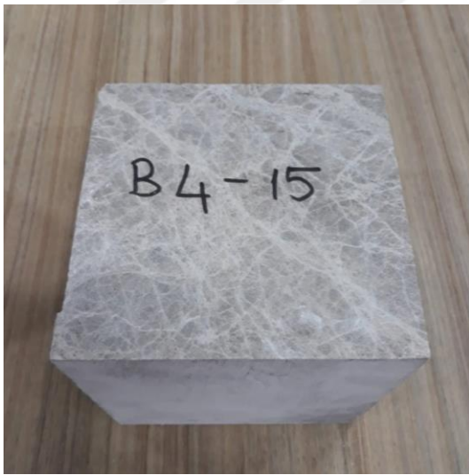
Figure 4.26. Pre-thermal damage-B4-15 (at 0°C)
