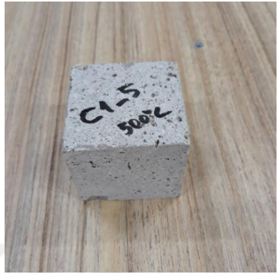
Figure 4.73. Post-thermal damage-C1-5 (at 500°C)
