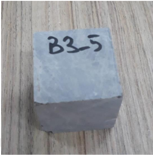
Figure 4.68. Pre-thermal damage-B3-5 (at 0°C)
