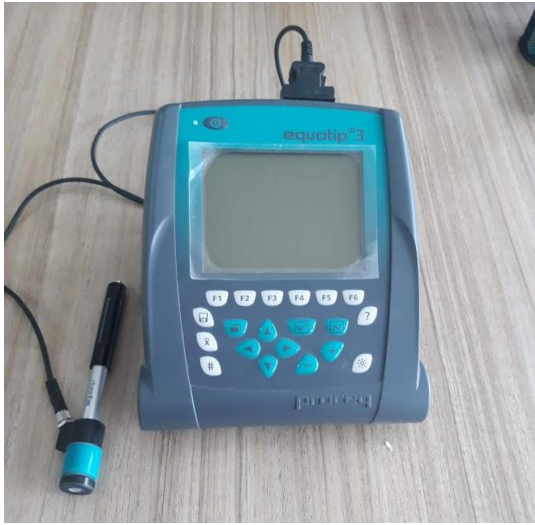
Figure 3.6. Proceq Equotip Portable Hardness Tester
