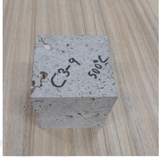
Figure 4.53. Post-thermal damage–C3-9 (at 500°C)
