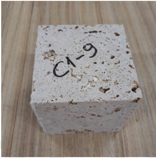
Figure 4.48. Pre-thermal damage–C1-9 (at 0°C)
