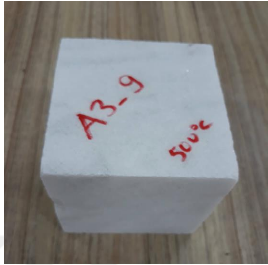
Figure 4.37. Post-thermal damage–A3-9 (at 500°C)
