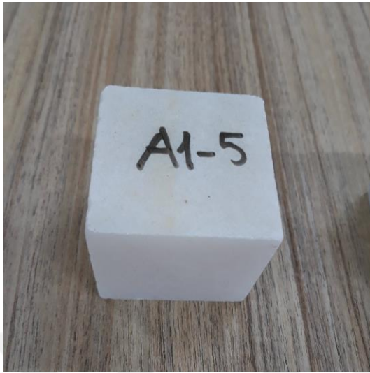
Figure 4.56. Pre-thermal damage–A1-5 (at 0°C)
