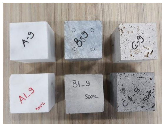
Figure 4.100. Samples pre- and post-thermal damage tests (A-9, B-9, C-9 at 0°C and A1-9, B1-9, C1-9 at 500°C)
