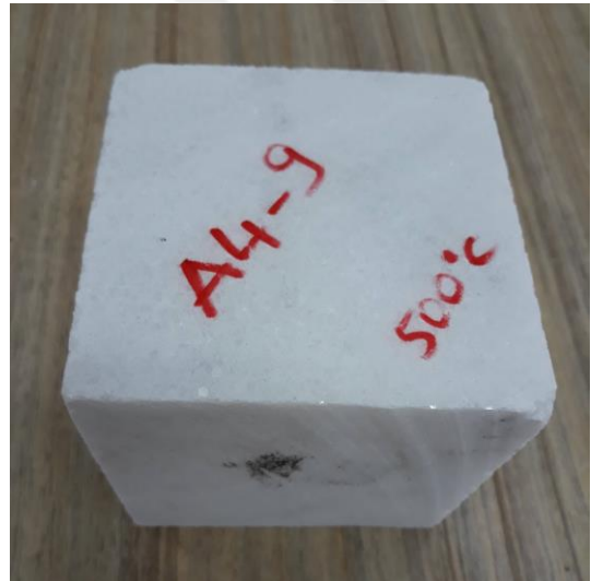
Figure 4.39. Post-thermal damage–A4-9 (at 500°C)
