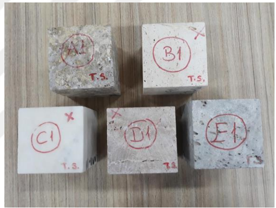
Figure 4.99. Samples subjected to thermal shock tests (at 100°C)
