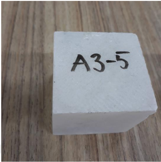
Figure 4.60. Pre-thermal damage–A3-5 (at 0°C)
