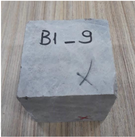
Figure 4.40. Pre-thermal damage-B1-9 (at 0°C)
