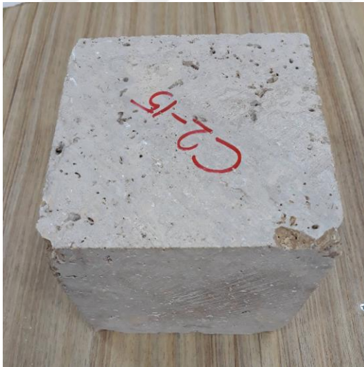
Figure 4.30. Pre-thermal damage–C2-15 (at 0°C)
