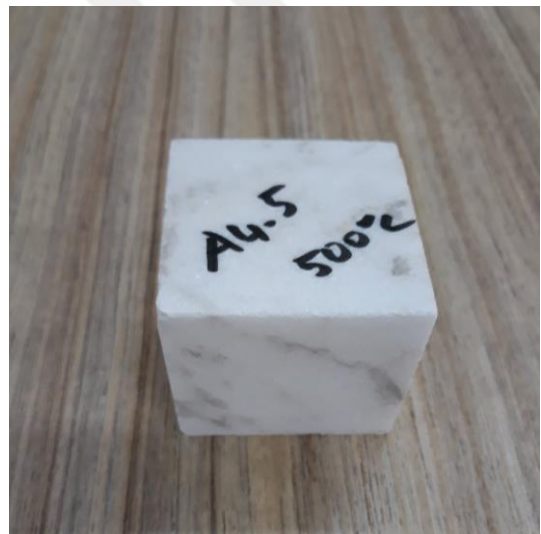
Figure 4.63. Post-thermal damage–A4-5 (at 500°C)
