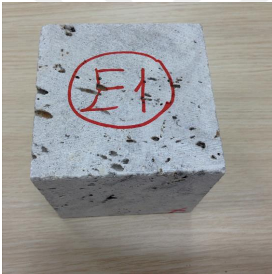
Figure 4.5. Thermal shock – Sample E1
