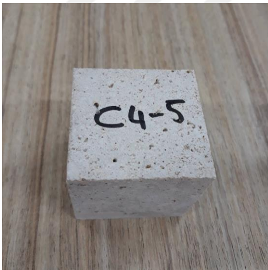
Figure 4.78. Pre-thermal damage–C4-5 (at 0°C)
