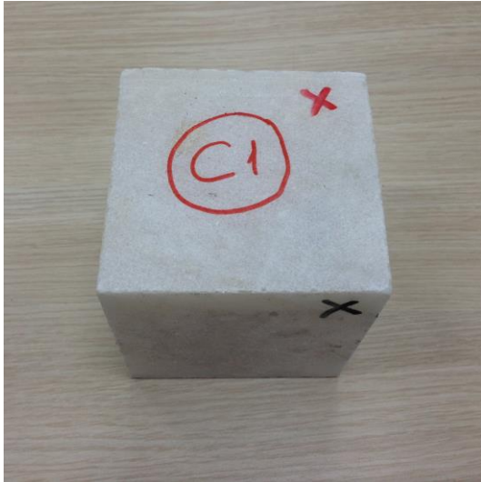
Figure 4.3. Thermal shock – Sample C1
