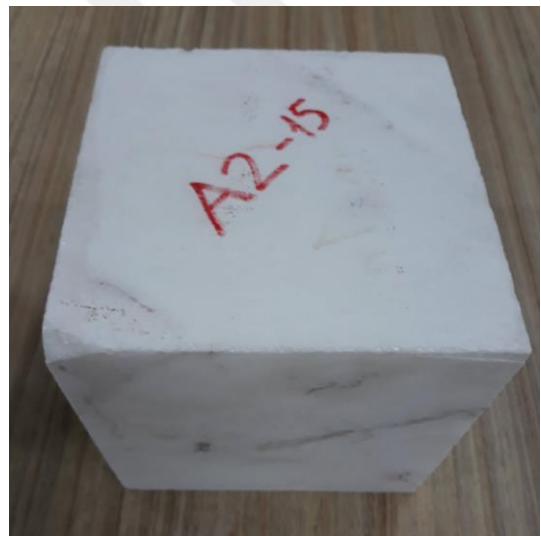
Figure 4.15. Post-thermal damage–A2-15 (at 500°C)
