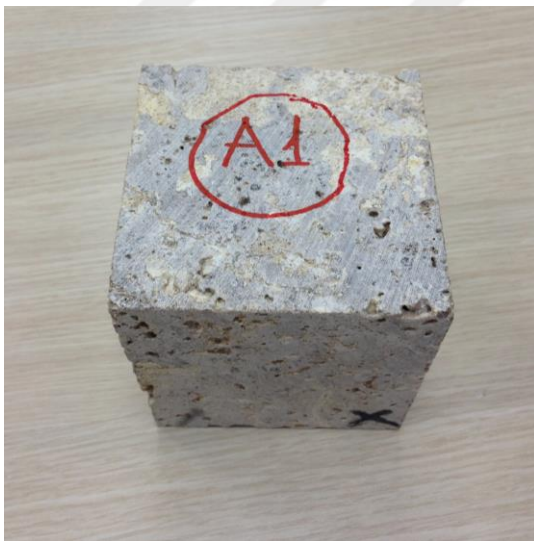
Figure 4.1. Thermal shock – Sample A1
