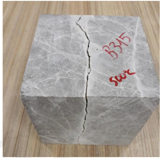
Figure 4.25. Post-thermal damage-B3-15 (at 500°C)
