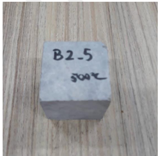
Figure 4.67. Post-thermal damage-B2-5 (at 500°C)
