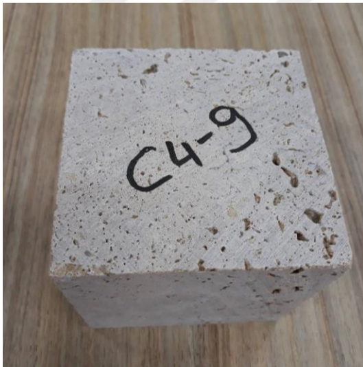
Figure 4.54. Pre-thermal damage–C4-9 (at 0°C)
