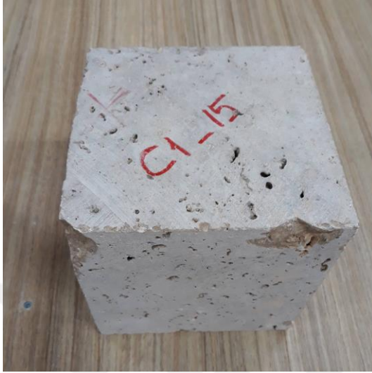
Figure 4.28. Pre-thermal damage–C1-15 (at 0°C)
