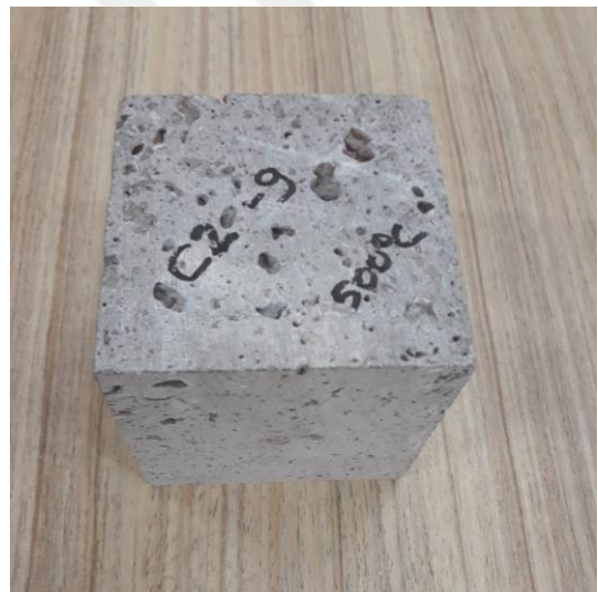
Figure 4.51. Post-thermal damage–C2-9 (at 500°C)
