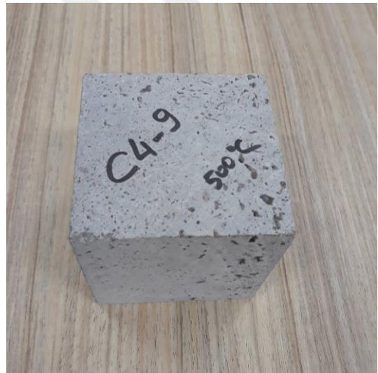
Figure 4.55. Post-thermal damage–C4-9 (at 500°C)
