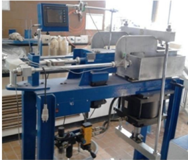
Figure 2.20. Photography of direct shear test setup (Naeni and Gholampoor, 2018)
