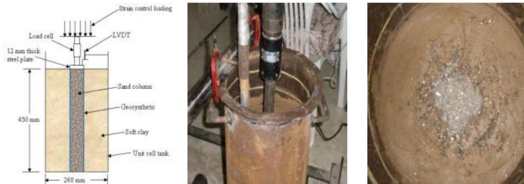
Figure 2.12. Schematic view and test set up by (Tandel et al., 2012)
