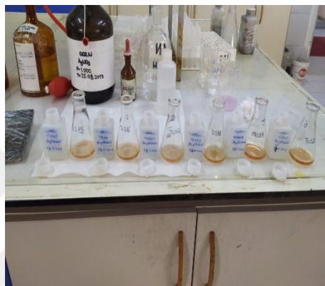
Figure 2.9. During free cyanide analysis the color change after dropping silver nitrate prepared solution
