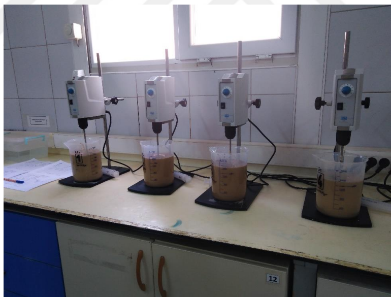
Figure 2.6. Tank (Agitation) Leach Test Assembly
