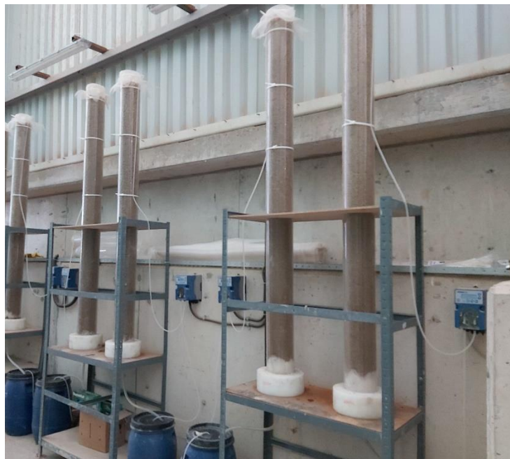
Figure 2.4. Column Test Assembly (1st group column tests)
