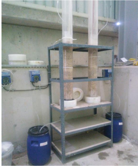
Figure 2.5. Column Test Assembly (2nd group column tests)
