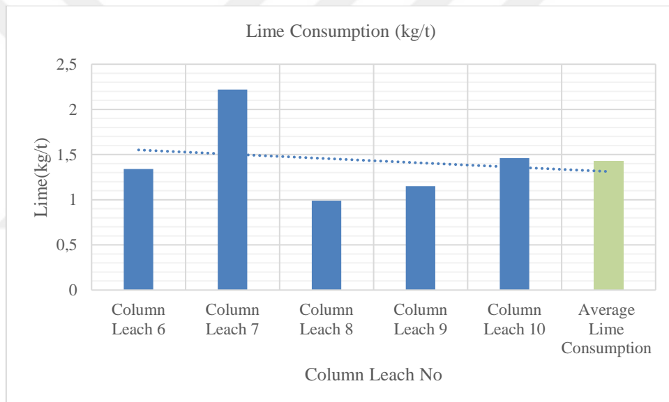
Figure 3.33. Lime Consumption for column fine particle size
