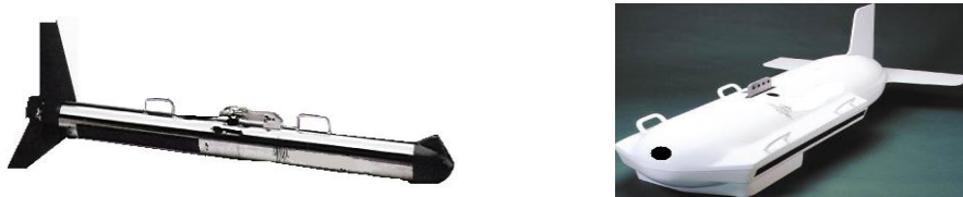
Şekil 2.5: (a) SIS 1500 Towfish, (b) Benthos TowFish -TTV -190 [29]
