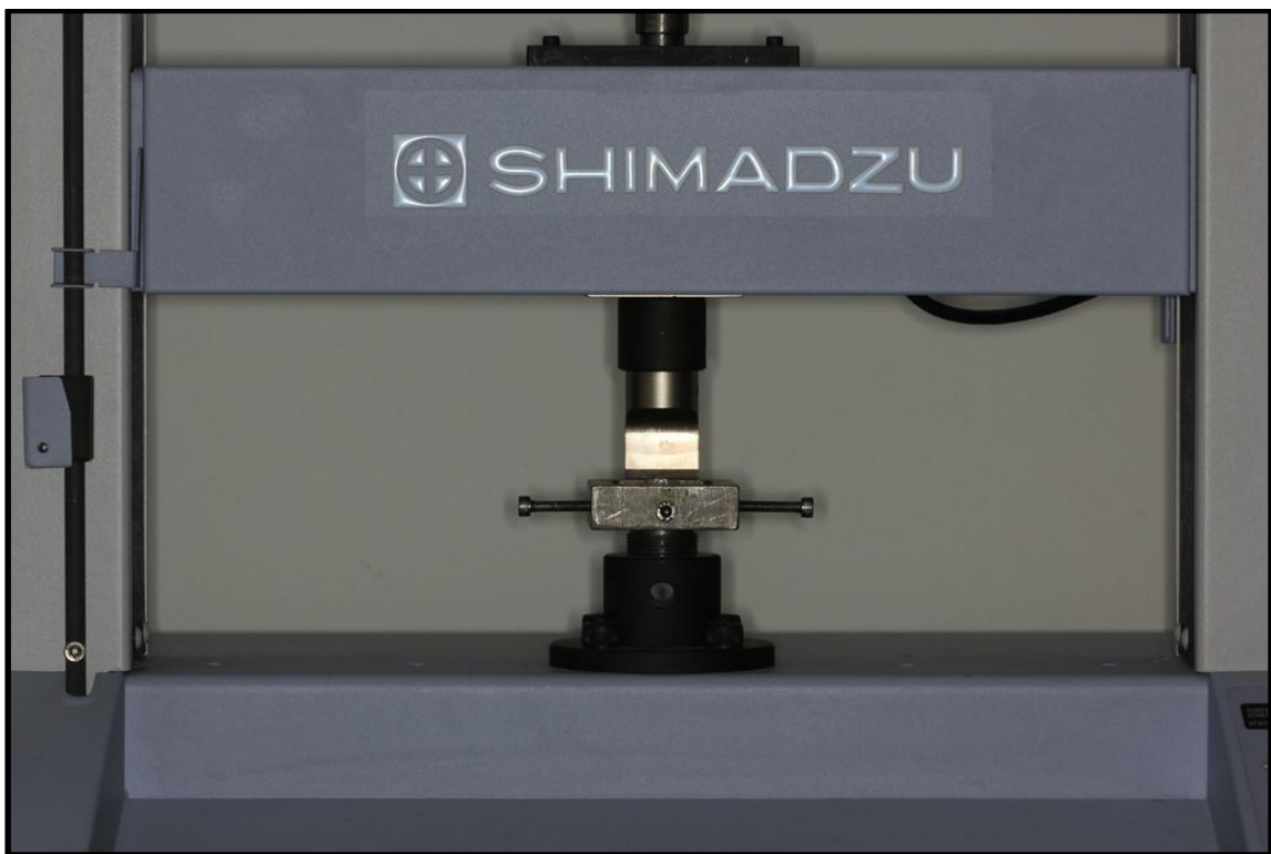
Figure 3.13 Debonding procedure using Universal testing machine
