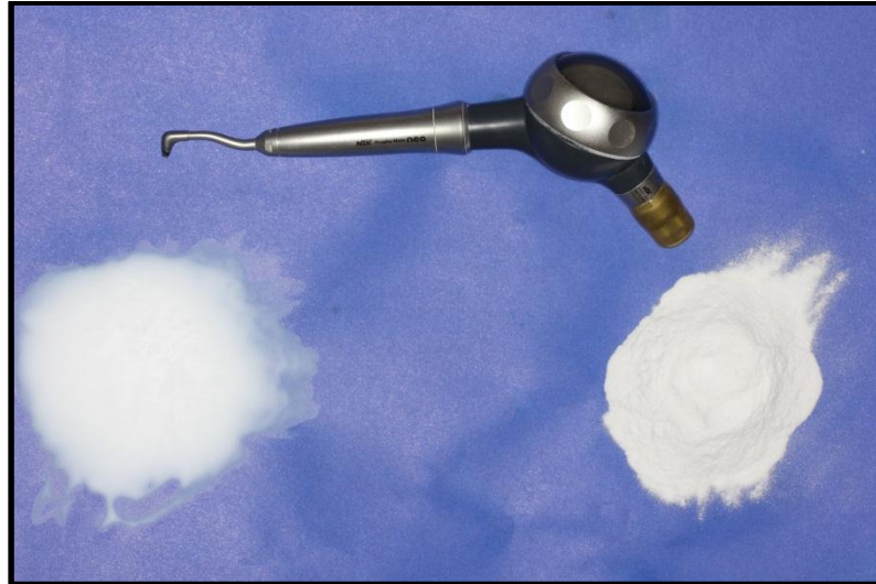
Figure 3.5 Blasting Materials (on the left side Silicon dioxide, on the right side Aluminum oxide)
