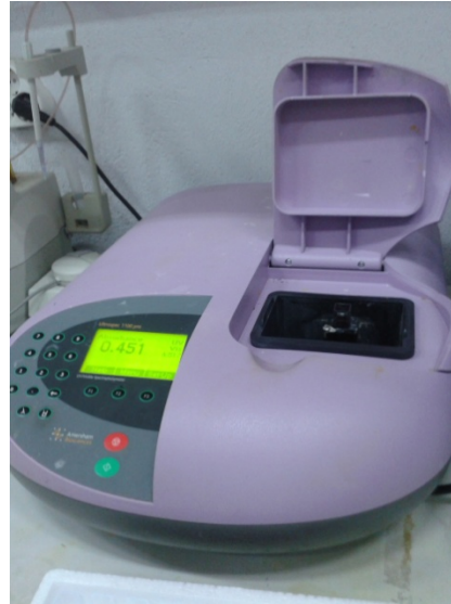
Şekil 2.7. Amersham Pharmacia Ultrospec 1100 Pro UV/ Visible Spectrophotometer
