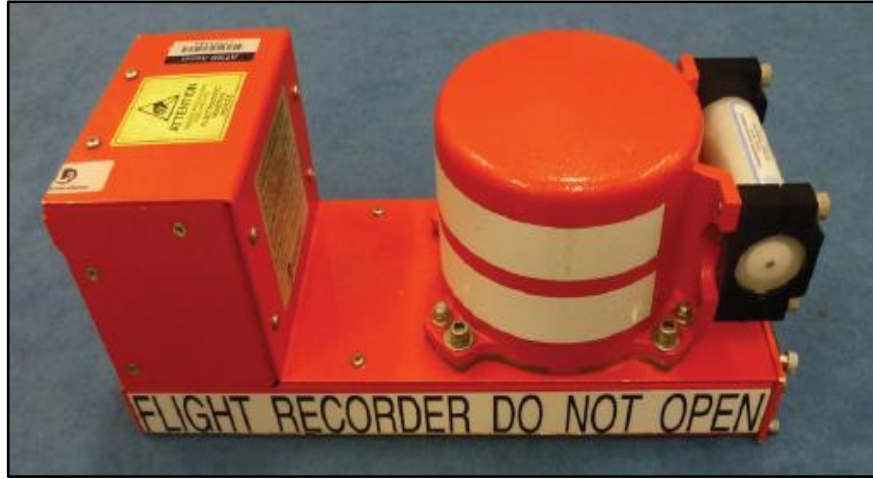
Şekil 2.2. Cockpit Voice Recorder (CVR) [34]
