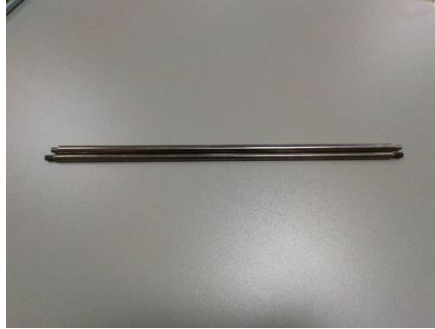
Figure 2.3. Steel bars for main and tail beam
