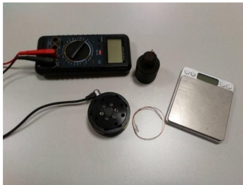
Figure 3.5. Components for static torque and force testing
