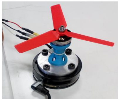
Figure 3.8. Static test setup for torque measuring
