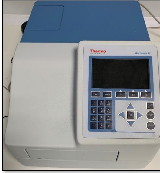
Resim 21. ELISA mikroplate optik okuyucu. (Multiskan™ FC Microplate Photometer, Thermo Fisher Scientific, Madrid, İspanya)
