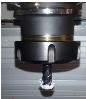
Figure 4.1. The welding of the workpiece on the carbide tool in dry machining
