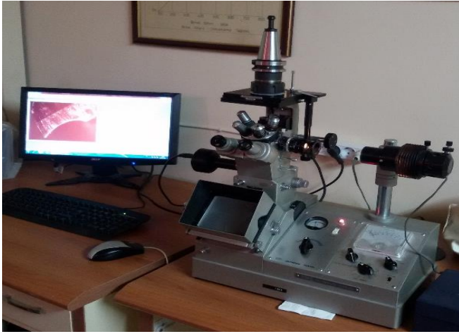
Figure 3.7. Measurement of tool wear
