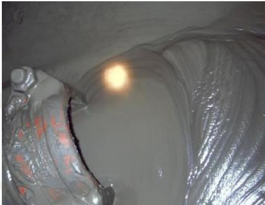
Figure 3.14. Hydraulic fill – Model 1 (O'Toole et al., 2011)
