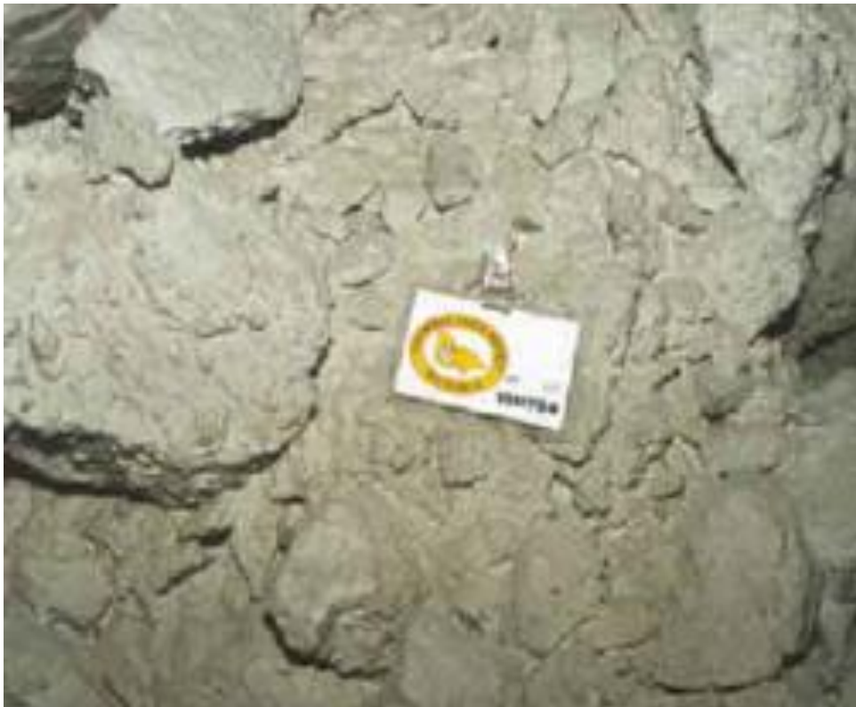
Figure 3.15. Cured cemented rock fill– Model 2 (Dorricott and Grice, 2002)
