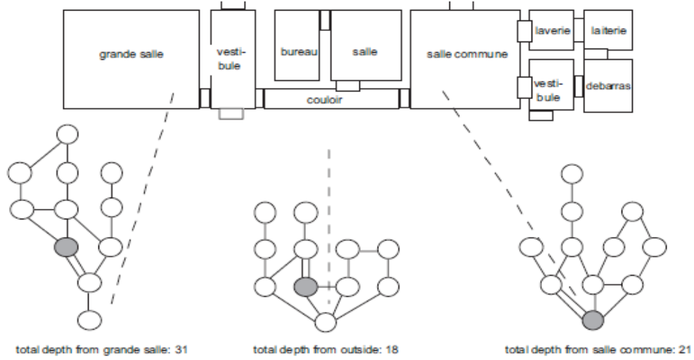
Fig. 3. The layout of a house looks more, or less, integrated from different points of view.
