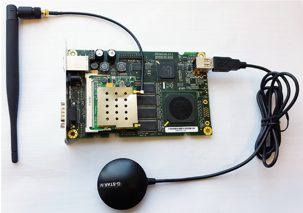
Figure 3.6 Prototype with Alix3D2 development board.
