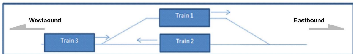
Figure 3.2 Feasibility will be guaranteed by forcing Train 3 to wait without entering the station until Train 1 leaves the station.
