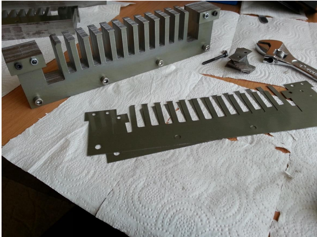
Figure 4.3 Silicon steel lamination and package of motor
