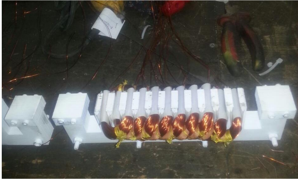
Figure 4.4 Painted core with motor coils
