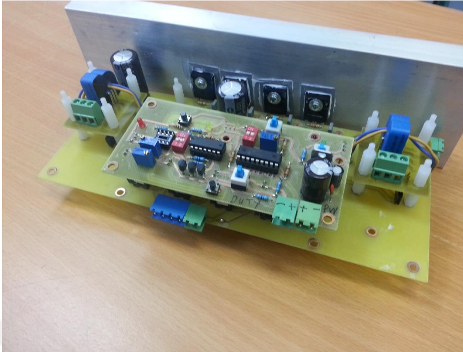
Figure 4.11 One phase 1kW motor driver
