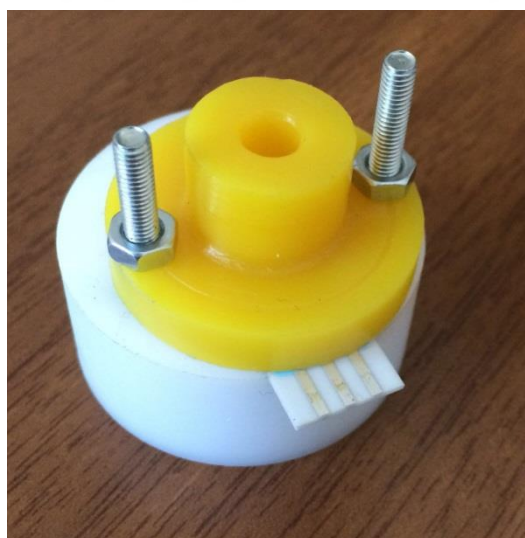
Figure 3.4 Designed tool for thiol modification of gold working electrode area
