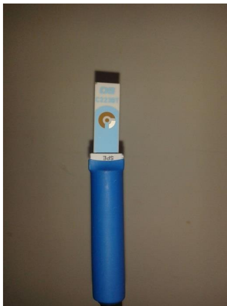
Figure 3.3 SPGE which is conducted by conductor cable
