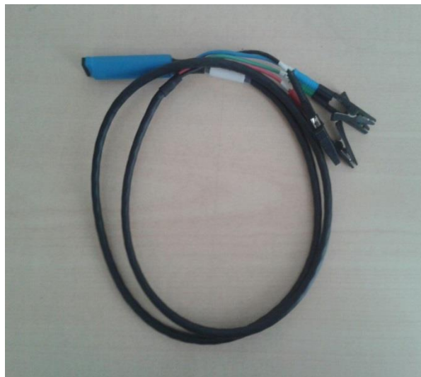
Figure 3.2 Conductor cable for conductance of SPGE and potansiostat/galvonastat device
