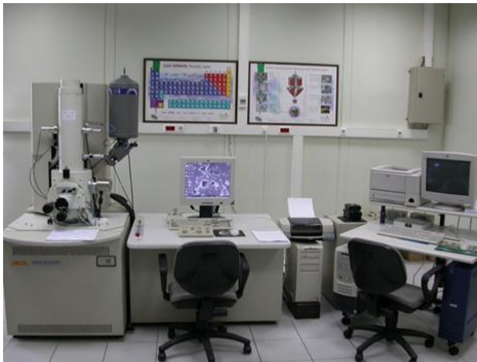
Figure 2. 8 Jeol JSM 6335F Field Emission Scanning Electron Microscope used for investigating the internal morphologies of dried gels
