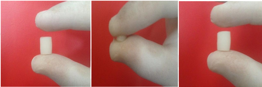
Figure 3. 10 The digital images swollen 5 w/v % OVA with 1 w/v % HA biocomposite cryogels when being squeezed between fingers
