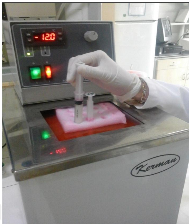
Figure 2. 6 The incubation of the gels in the cryostat at -12^{\circ}\text{C}
