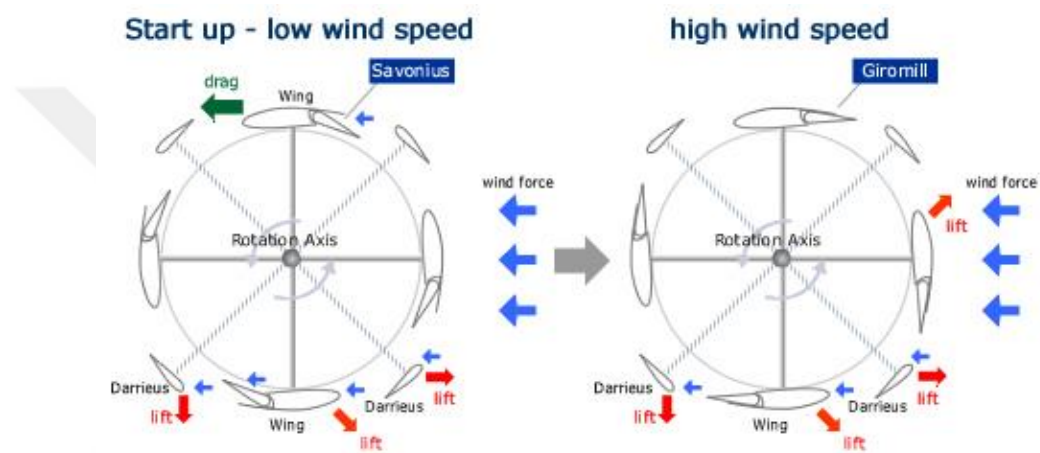
Figure 2.3 Lift Mechanism of Darrieus Style Wind Turbine blade
