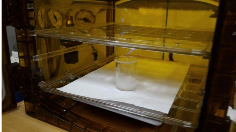
Figure 2.50 Emptying the air inside the PDMS with the desiccator
