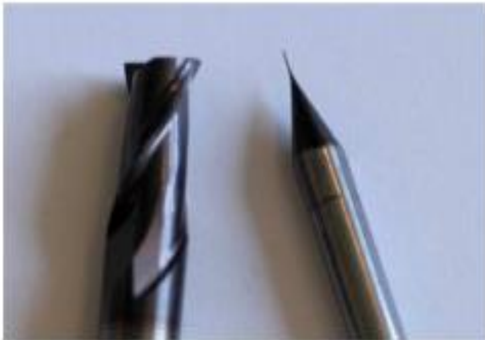
Figure 2.23 Micromechanical machining precision and micro-finger milling pocket with a diameter of 6mm - 200 microns
