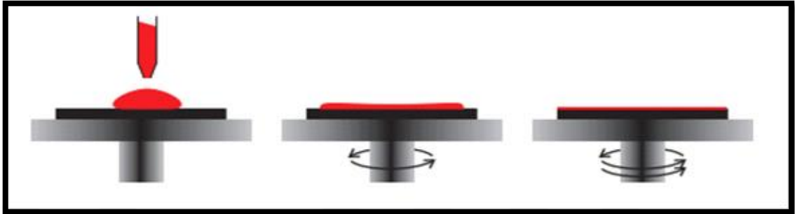
Figure 2.45 Spin coating working principle[25]
