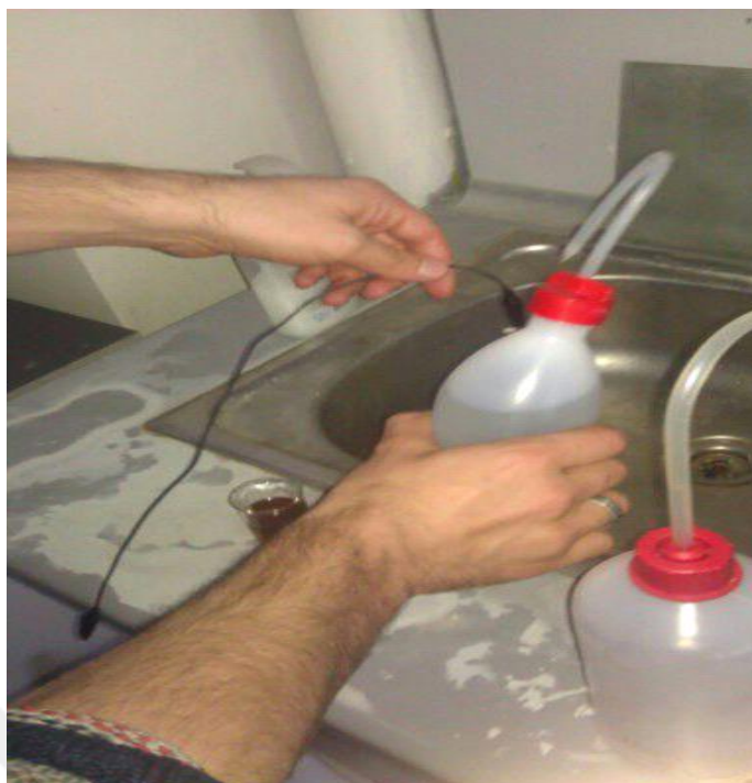
Figure 2.29 Preparation of Diluted HCl Solvent for Polymeric Material Cleaning
