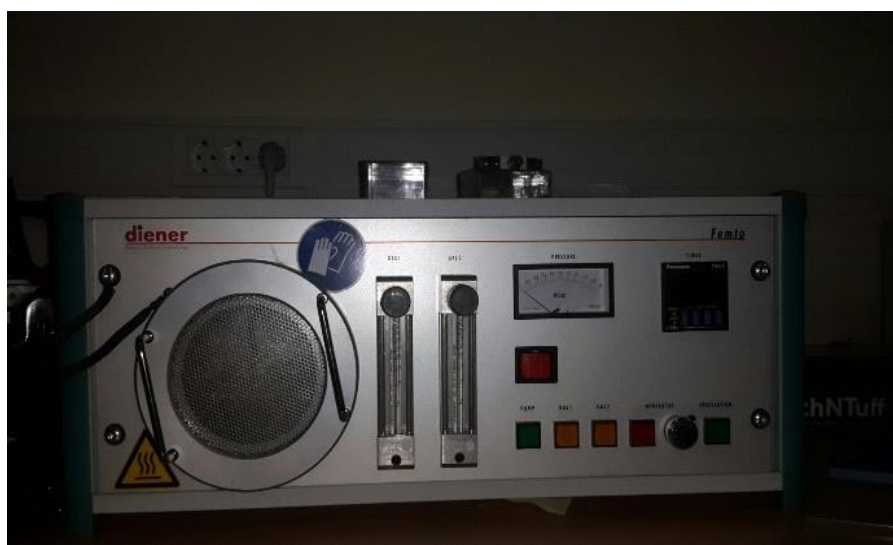
Figure 2.55 Plasma apparatus used for bonding PDMS with glass slide
