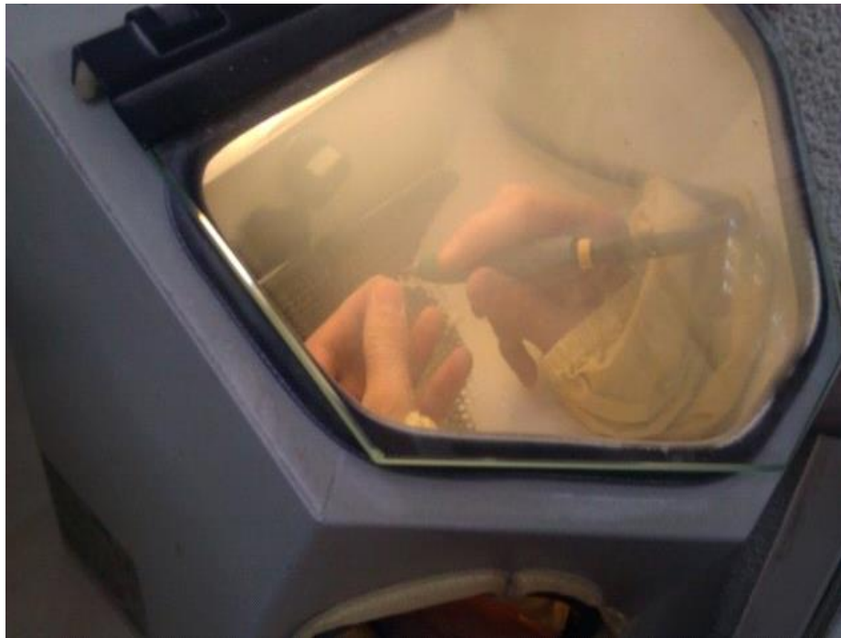
Figure 2.21 Glazing process to reduce burrs and cavities of Nickel-based Microrobot produced by laser cutting
