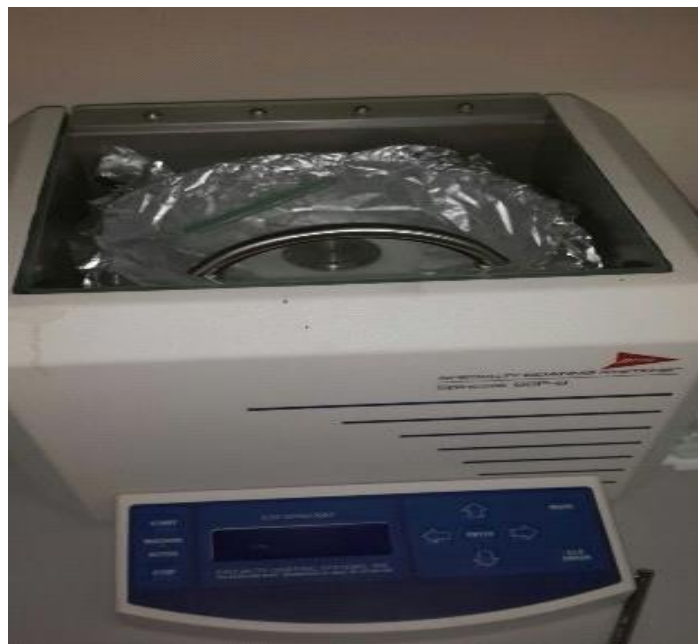
Figure 2.46 Spin coater used in coating of photoresist on wafer in Central Laboratory
