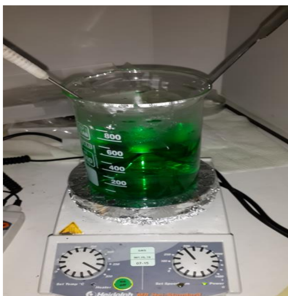
Figure 2.35 Coating of the polymer micro-robot arm in a current-free nickel plating chamber at 80 ° C
