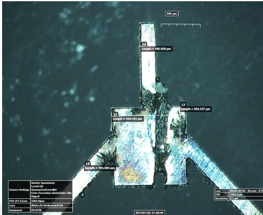
Figure 2.18 First Nickel-Based Micro-Robot Arm Produced by Laser Cutting
