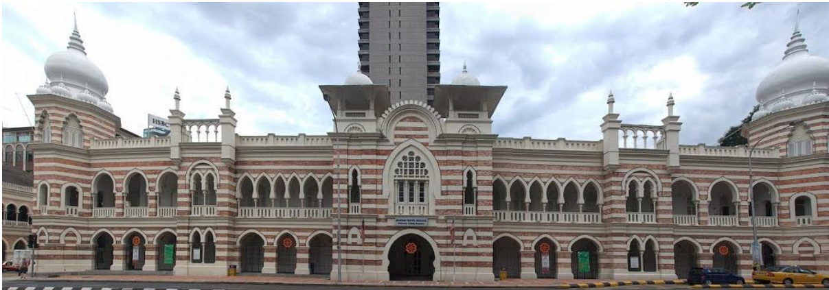
Figure 4.95 A range of multifoil arches, horseshoe arches and pointed horseshoe arches at former FMSR Headquarters, Kuala Lumpur Malaysia
