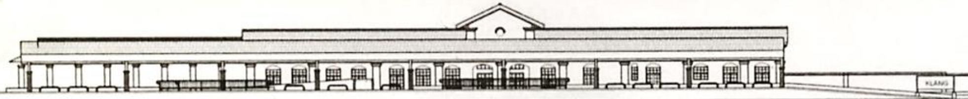
2. Rear Elevation shows the façade from the tracks with series of casement windows, [78]
