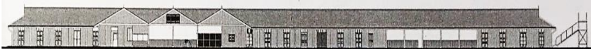
1. Rear Elevation shows the façade from the tracks with three gable roof intersecting with main hip gable roof [67]
