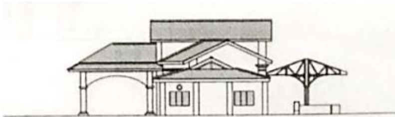
3. East Elevation shows the entrance porch, main building and its platform with train-shed, [78]
