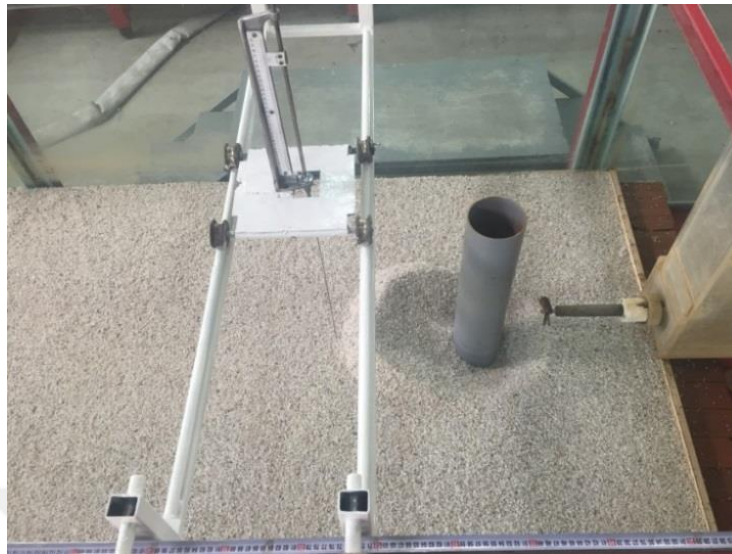
Figure 6.31 Scour profile measurements by using a limnimeter
