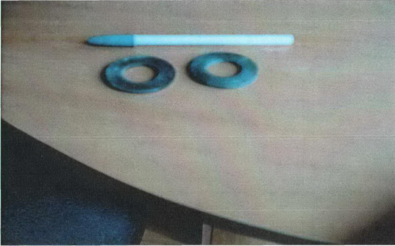
Figure 2.3. Polycarbonate samples in ring shape
