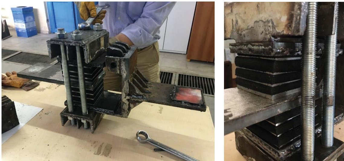
Figure 4.16 Squeezing the nuts after the first phase
