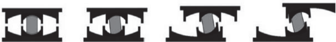
Figure 2.4 Different stages during the displacement of a triple pendulum bearing [3]
