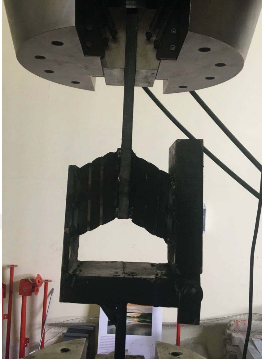
Figure 4.8 Deformation along shear direction
