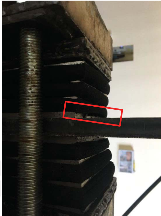
Figure 4.15 Bonding Failure during the first phase
