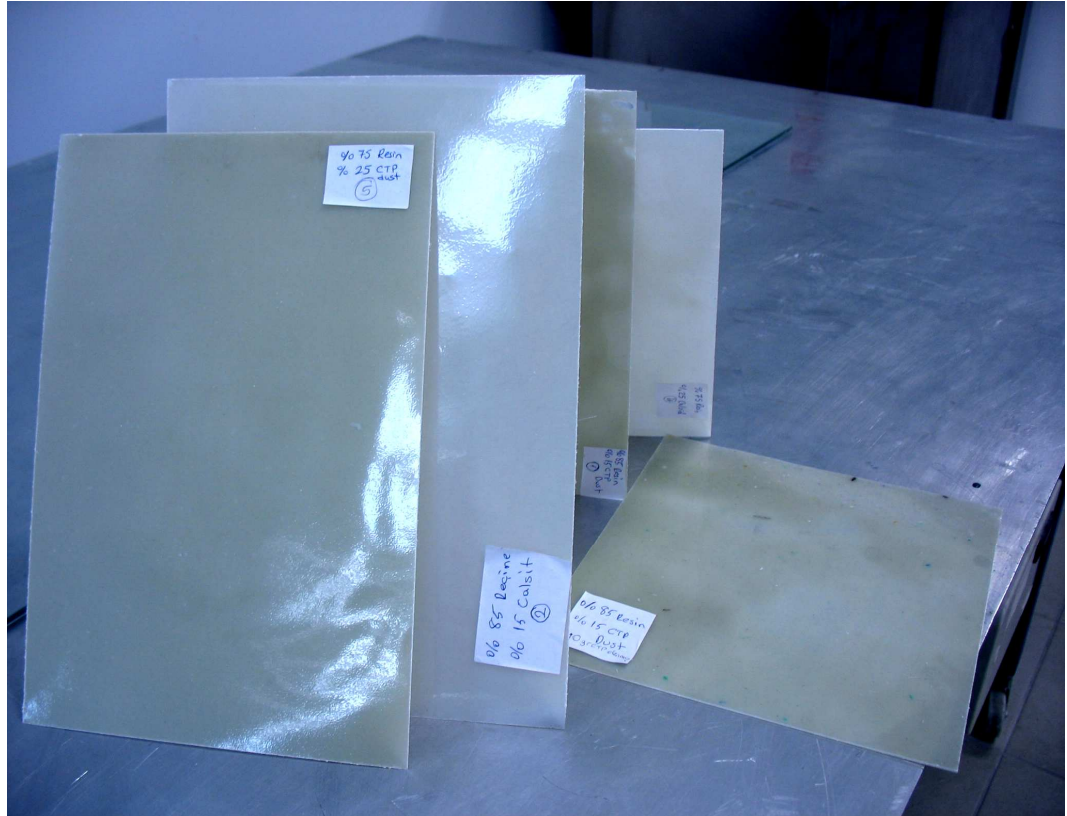
Figure 2.7 The experimental GRP composite sheet samples after hand layup process
