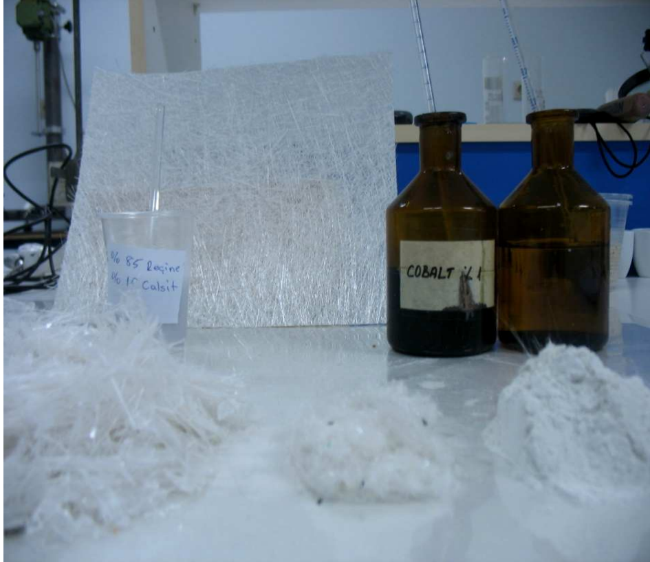
Figure 2.5 Experimental set up for hand lay up proces in Fibrosan laboratory, Izmir
