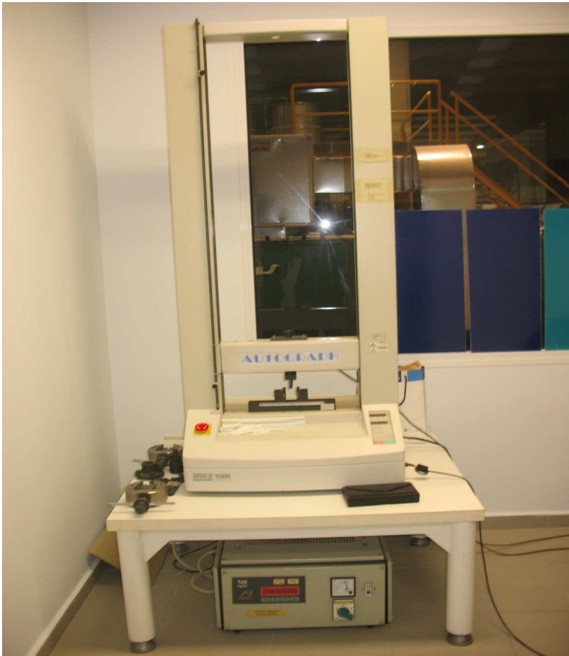
Figure 2.6 The AGS-J Shimadzu Autograph Flexural test machine
