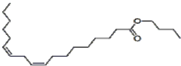
Figure 2.3.1 Chemical chain structure of linoleic acid butyl ester
