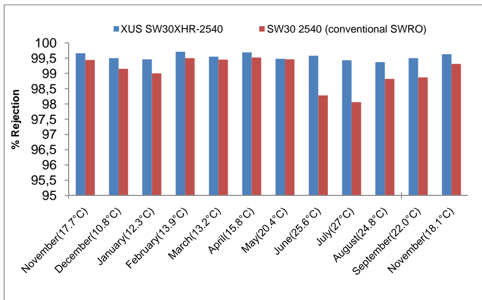
Figure 3.61 Variations in \text{Na}^+ rejections of permeate during one year of operation (Tests 3, 6, 9, 10, 12, 15, 16, 18, 19, 20, 22 and 23)
