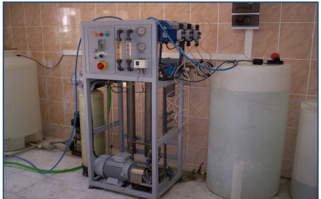
Figure 2. 1 Reverse osmosis system at Urla, İZMİR
