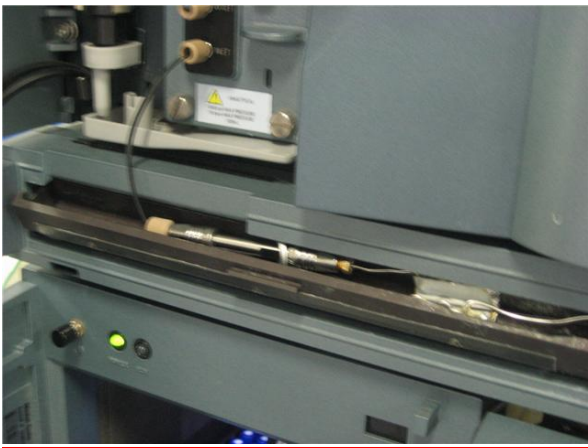
Figure 2.4. Column Manager out and detector in
