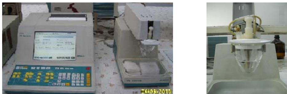
Figure 2.1. Metrohm 693 Voltammetric Analyzer (VA) processor and a 694 VA Stand with its own cell.
