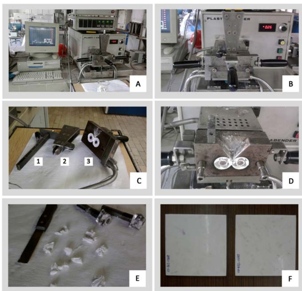
Figure 2.3 Composite production in the mixer. A: Overall set-up of computer controlled mixer, B: A closer view of mixing chamber, C: demounted state of the mixer; pushing part (1) feeding hopper (2) and outer cover (3), D: Mixer in open position, E: Mixing blades and produced pieces of composite, F: Compression molded composite samples.
