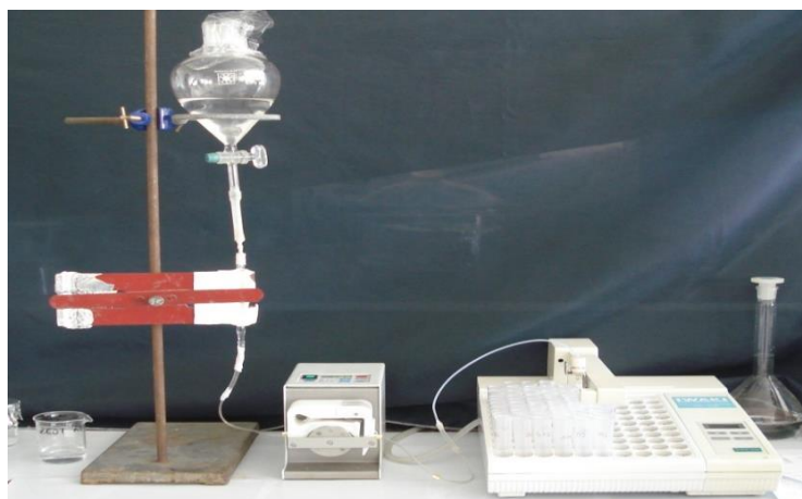
Figure 2.12. Experimental set-up of column-mode studies.
