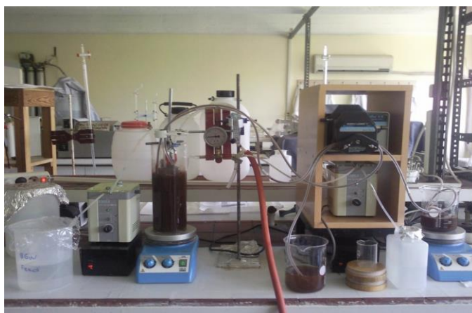
Figure 2.14. Experimental set-up of submerged sorption-membrane filtration hybrid method using lithium adsorbent.
