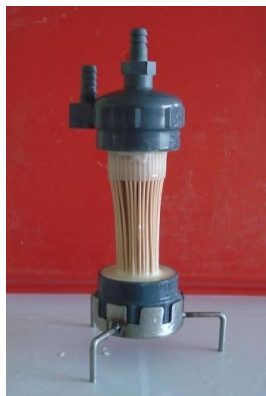
Figure 2.13. ZeeWeed ® -1 (ZW-1) hollow fiber ultrafiltration membrane module.
