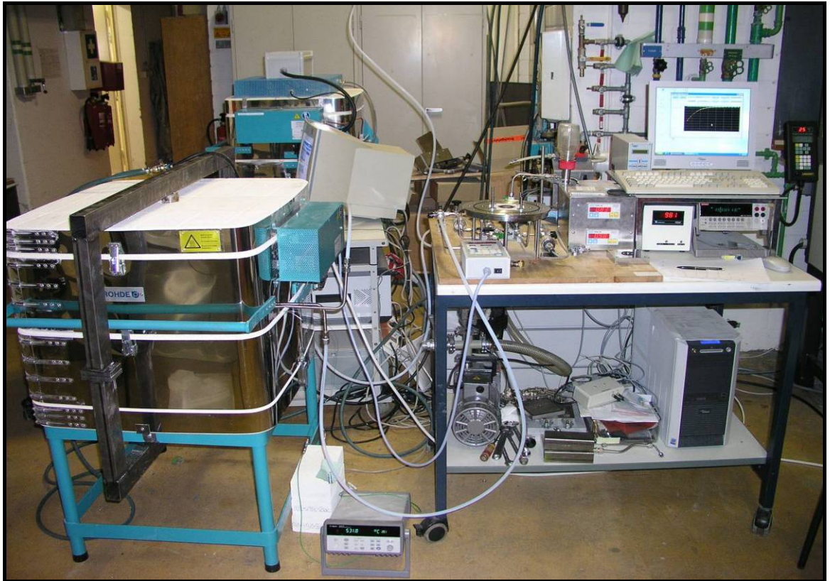
Figure 5.11 Leak rate measurement apparatus
