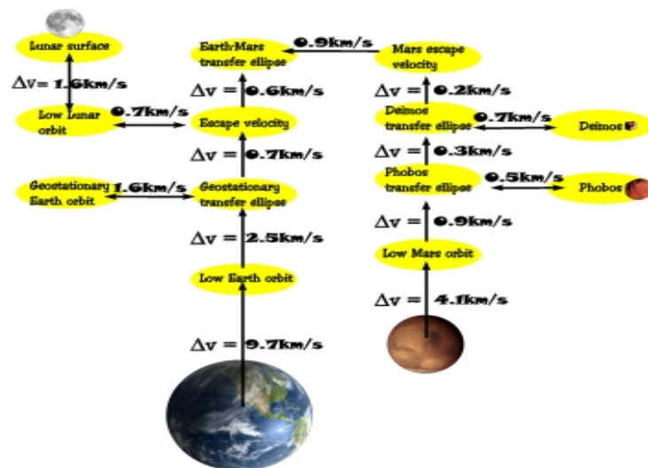
Figure 14.4 : Momentum Transfers in Mars Mission Using Nuclear Propulsion
