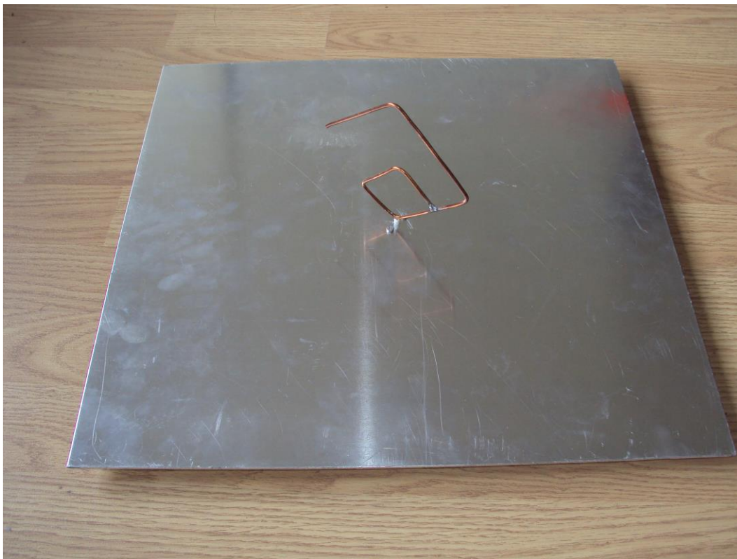
Figure 8.1 : Prototype antenna with L \approx 7.5 cm, radius = 1 mm
