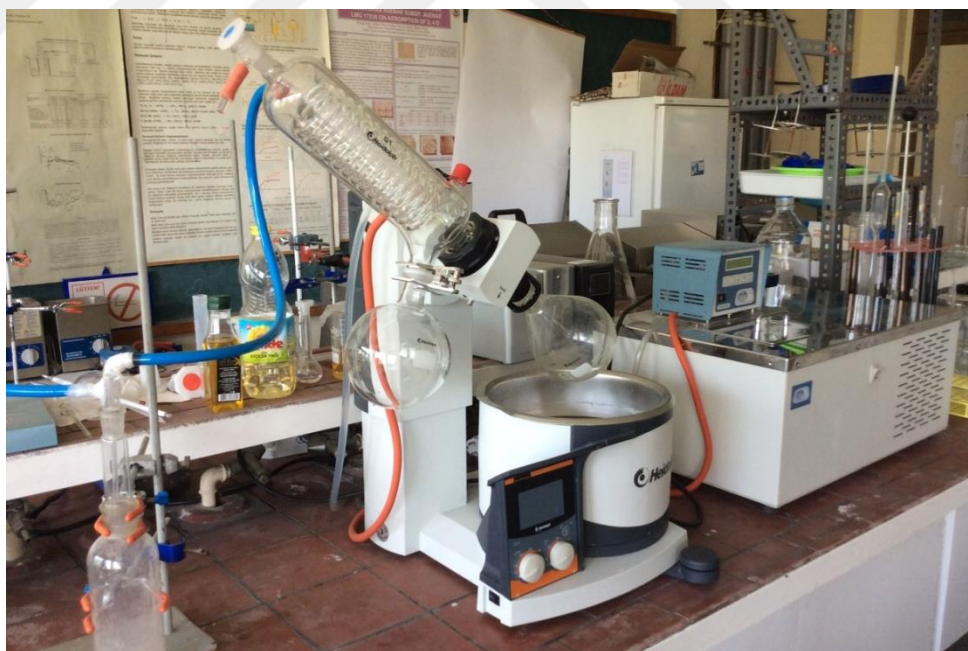
Figure 4.22. The utilized rotary evaporator (Hei-VAP series, Heidolph).
