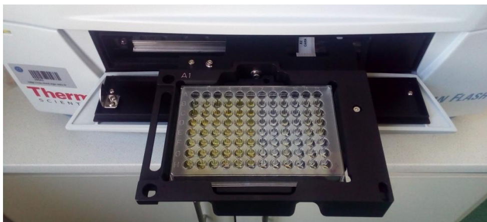
Figure 4.25. The microplate reader (Thermo Fischer, Varioskan Flash).
