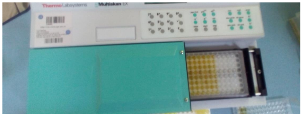
Figure 4.35. The Algae Extracts during Xanthine/xanthine oxidase Inhibition method. (Read in Thermo Labsystems, Multiskan EX)
