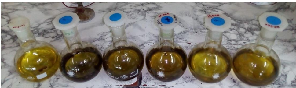
Figure 4.19. Varying light intensity (Increasing from left to right: 112, 174, 236, 275, 310, and 385 \mu\text{mol photon m}^{-2} \text{s}^{-1} respectively.
