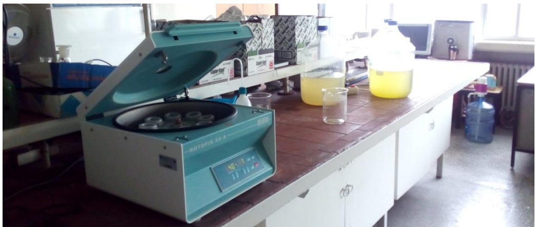
Figure 4.9. The centrifuge ( rotofix 32 A ) which was used throughout the study.
