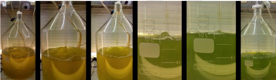
Figure 4.14. Growth at 385 \mu\text{mol photon m}^{-2} \text{s}^{-1} and 22^\circ\text{C} which had one of the highest biomass yields among the studied parameters, on days 1, 3, 5, 10, 15 and 21.
