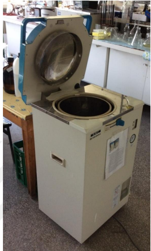
Figure 4.8. The Autoclave ( HMC HM 50-L ) which was used for sterilization during the study.
