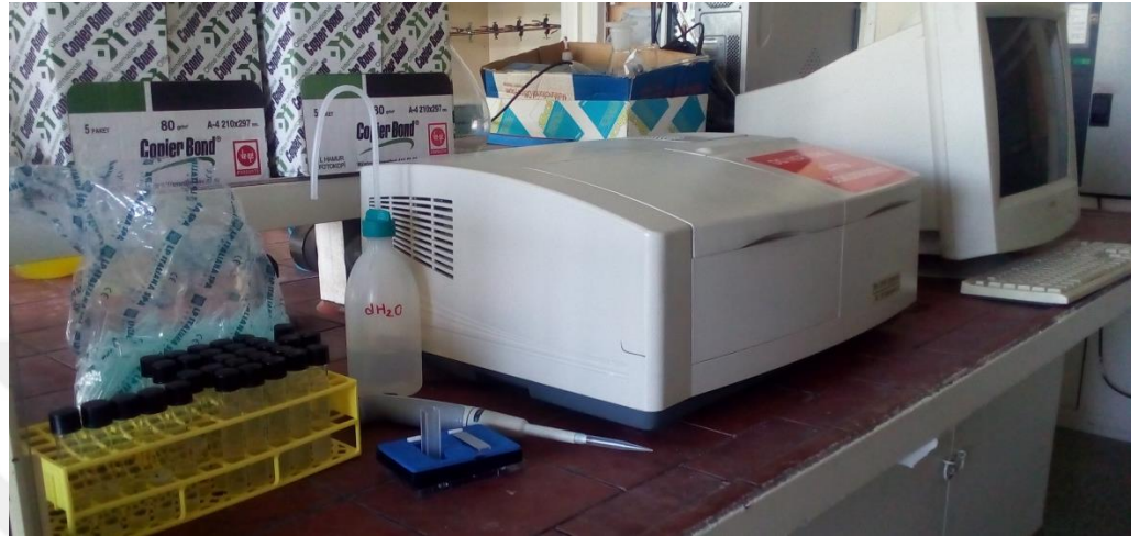
Figure 4.16. The Spectrophotometer ( T80+ UV/VIS Spectrophotometer ) Used for the Analyzes During Cultivation.
