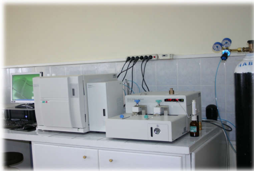
Figure 4-7. Total Organic Carbon Analyzer (SHIMADZU TOC-VCPH, JAPAN)
