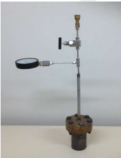
Figure 4-2. Batch SCWG system
