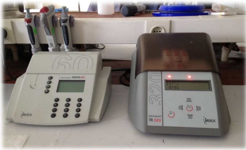
Figure 4-8. COD analysis equipments (thermo-reactor and spectrophotometer).
