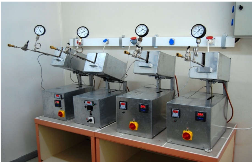
Figure 4-5. Batch autoclave reactors while the experiments are being performed.
