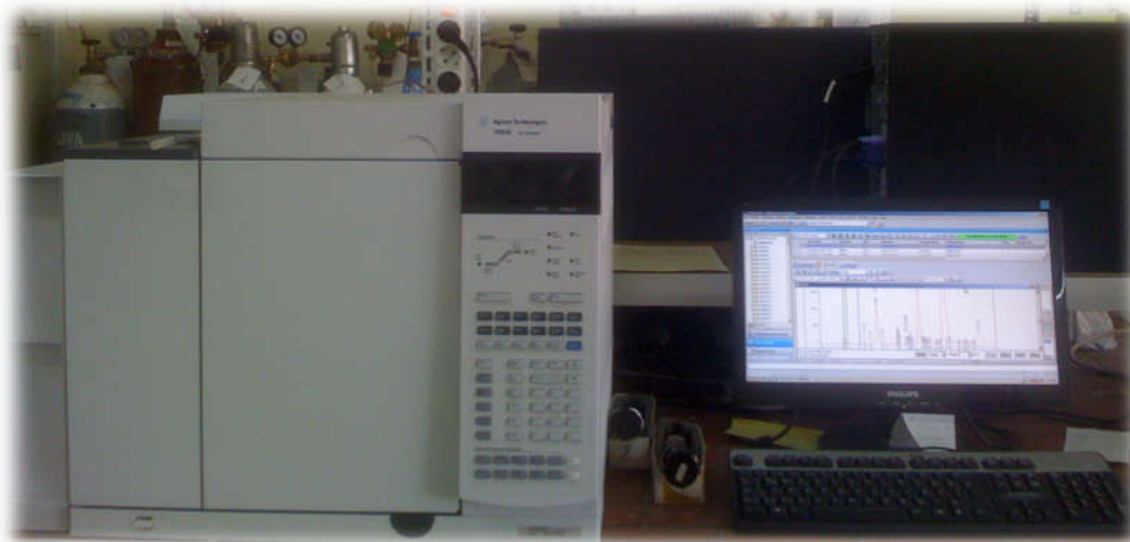
Figure 4-6. Gas Chromatography (AGILENT, GC 7890A) Gas Chromatography (AGILENT, GC 7890A)
