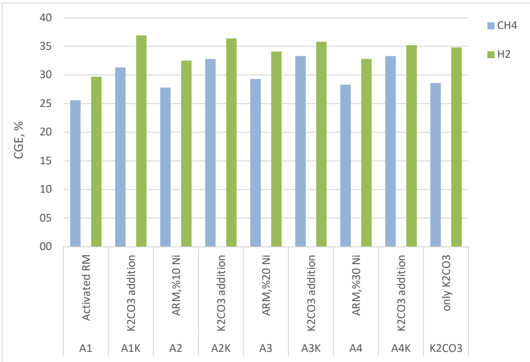
Figure 5-33. Effect of K 2 CO 3 addition and Nickel impregnation in A group catalysts on CGE.
