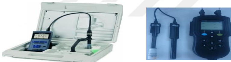
Figure 2.5. WTW pH 3110 pH-meter and Hach Lange HQ40d pH-meter
