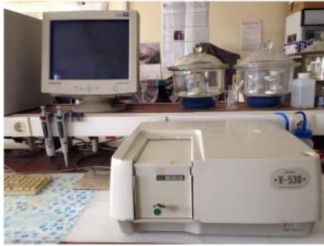
Figure 2.8. UV/vis spectrophotometer (Jasco V-530 model)
