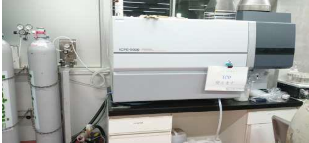
Figure 2.6. ICP-AES (Shimadzu ICPE-9000 Model with auto sampler ASC-6100)
