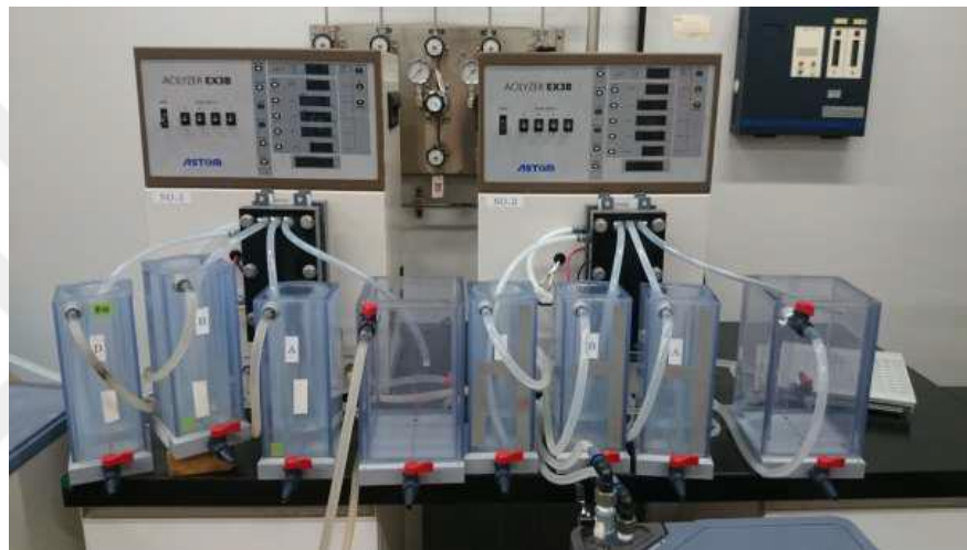
Figure 2.1. Astom Acilyzer EX3B model BMED system
