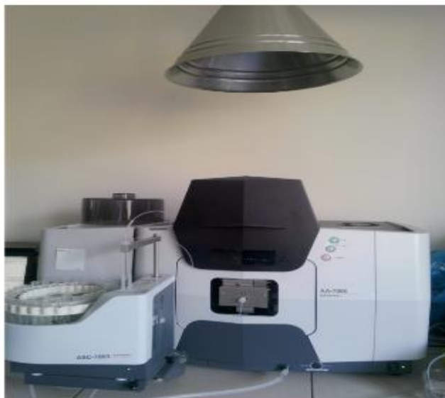
Figure 2.7. Atomic Absorption Spectrometer (Shimadzu AA7000 model AAS)
