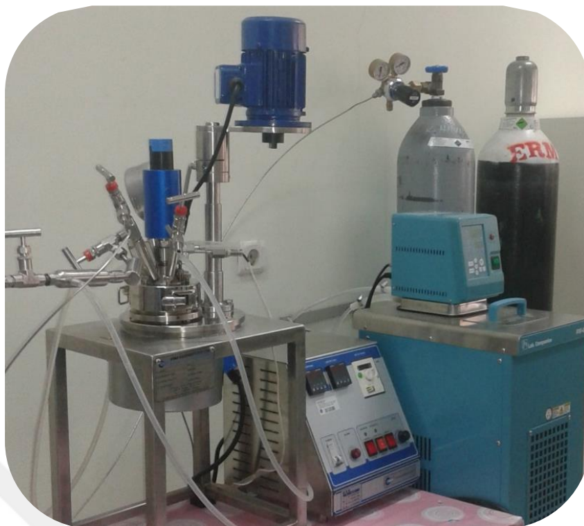
Figure5. 6 The high pressure stirred lab autoclave reactor system
