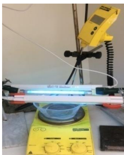
Figure5. 7 The picture of experimental setup for photocatalytic oxidation
