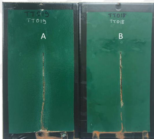
Figure 27 Salt Spray results of Coating A and B with scratch
