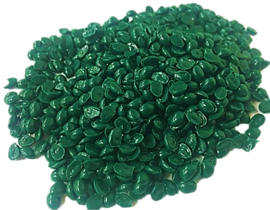
Figure 9 Plastic granules obtained from lab extruder - RAL 6005 color
