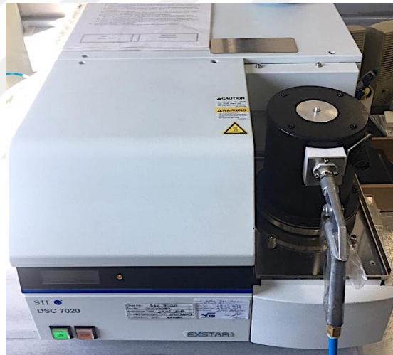
Figure 16 DSC Equipment - SII DSC 7020
