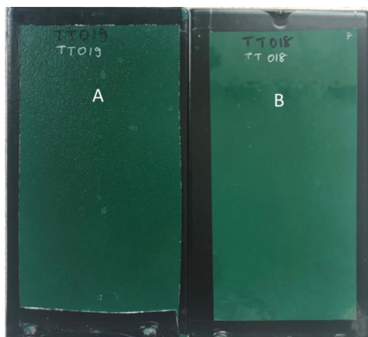
Figure 28 Salt Spray results of Coating A and B without scratch
