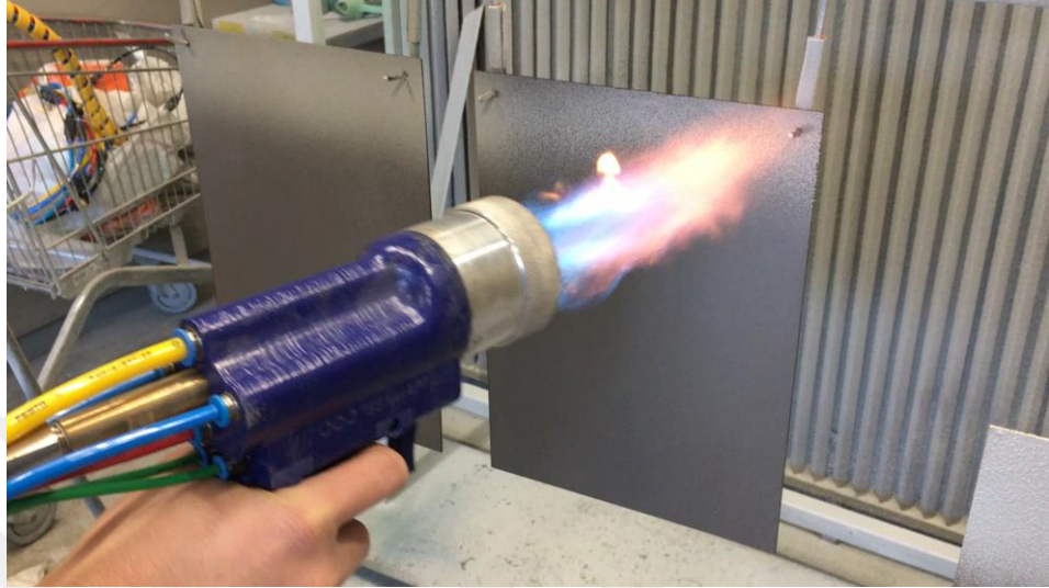
Figure 15 Flame Spray Application on a standard metal panels
