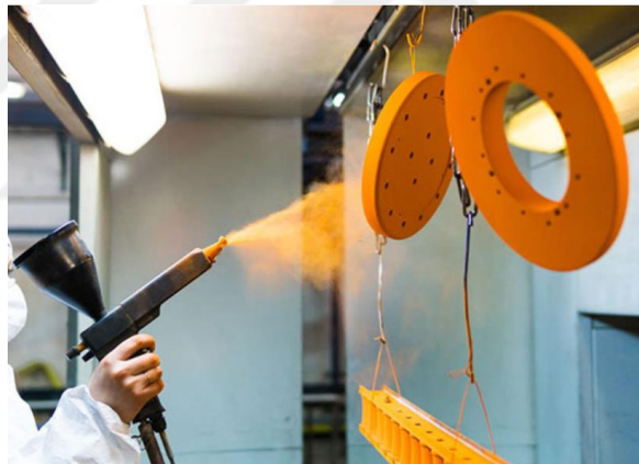
Figure 4 Electrostatic spray application of powder paint on metal objects
