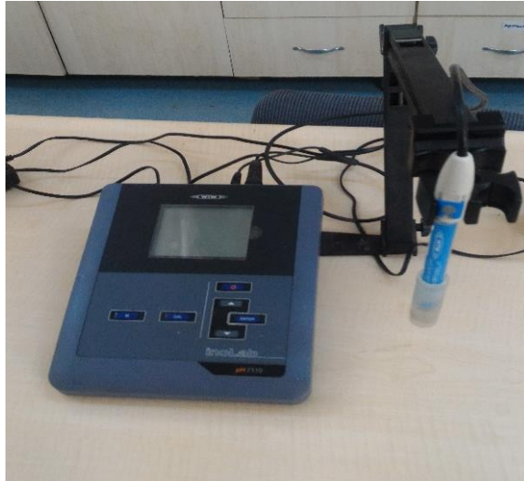
Şekil 3.13 Inolab marka pH level 7110 model (Almanya) pH metre
