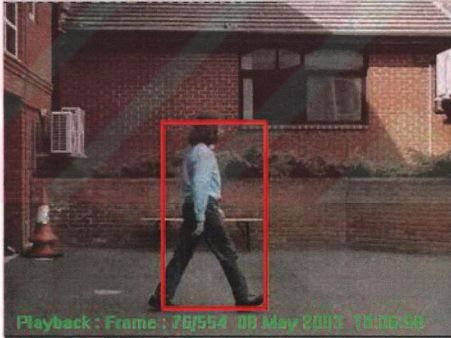
Figure 3.7: Minimum bounding box encapsulating the pixels classified as moving.
