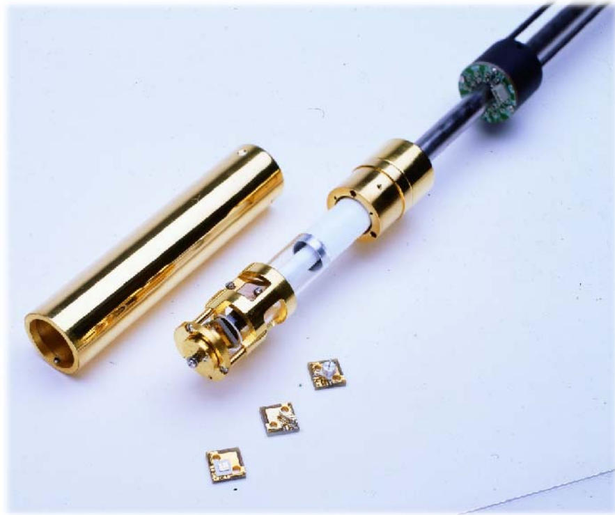
Figure 2.2: Picture of the microscope. The shield, puck & sample holder, slider glass and the piezos are shown.
