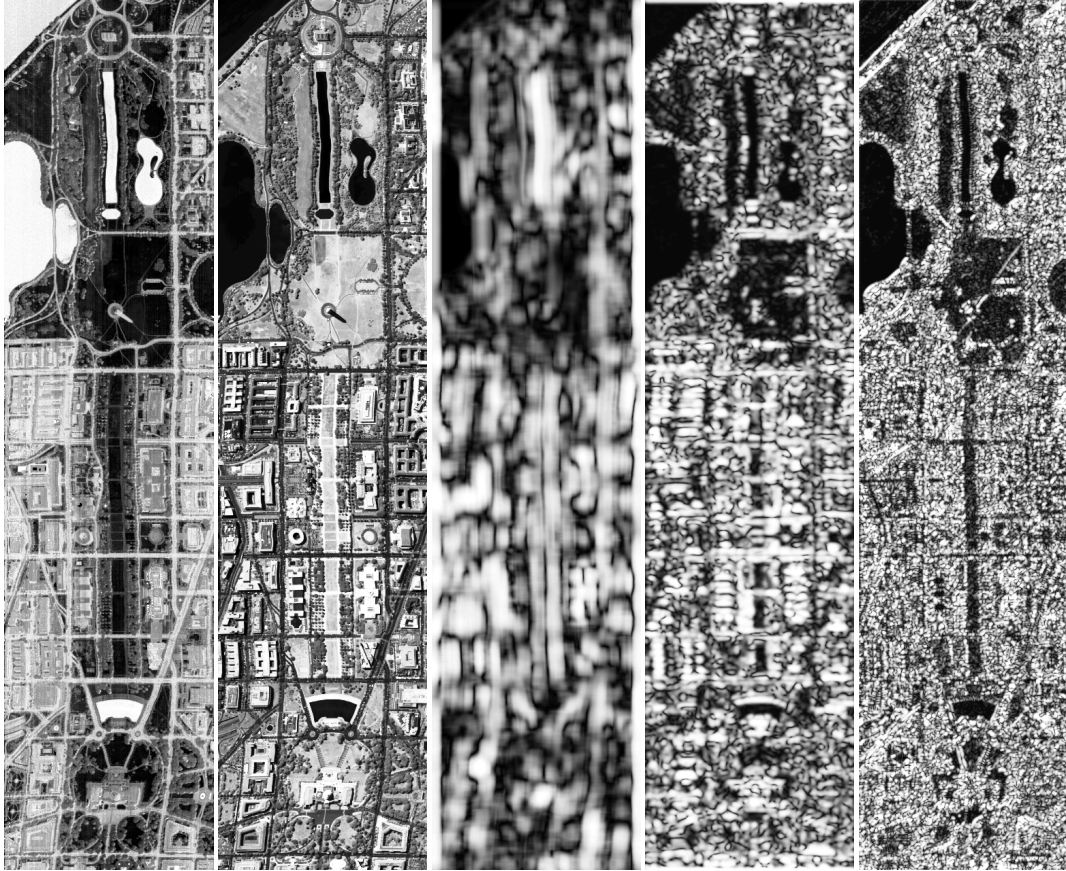
Figure 3.5: Pixel feature examples for the DC Mall data set. From left to right: the first LDA band, the first PCA band, Gabor features for 90 degree orientation at the first scale, Gabor features for 0 degree orientation at the third scale, and Gabor features for 45 degree orientation at the fourth scale. Histogram equalization was applied to all images for better visualization. (Images taken from [3].)
