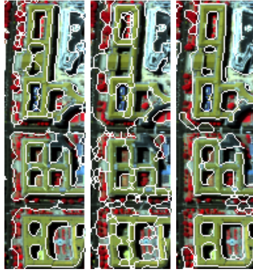
Figure 5.1: Example segmentation results (overlaid as white on false color and zoomed) for the DC Mall data set. The left, middle and right images show the extracted segments in the first, second and third PCA bands, respectively.
