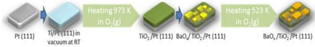
Figure 22. Sample preparation method for the BaO x films grown on TiO 2 /Pt (111) model system.
