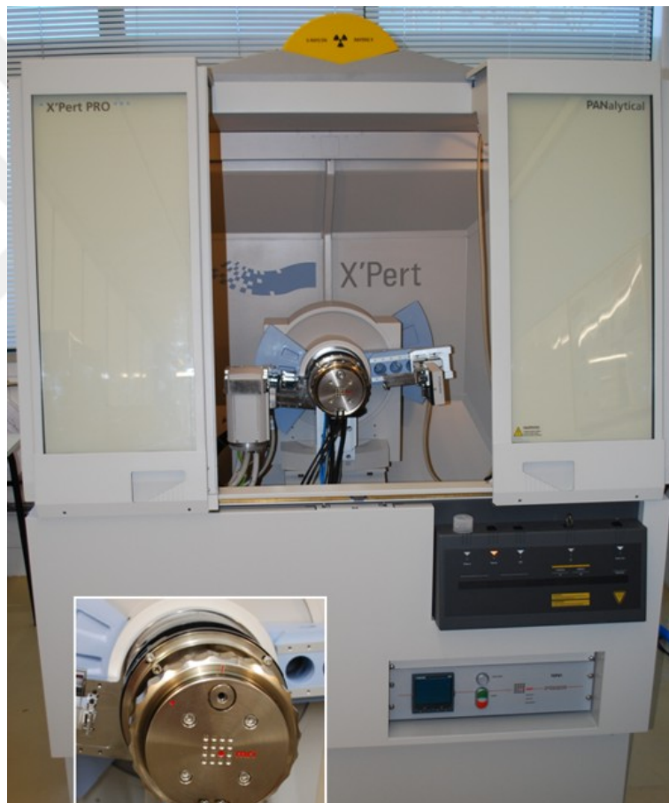
Figure 2.12: PANalytical's X'Pert PRO Materials Research Diffractometer [50]
