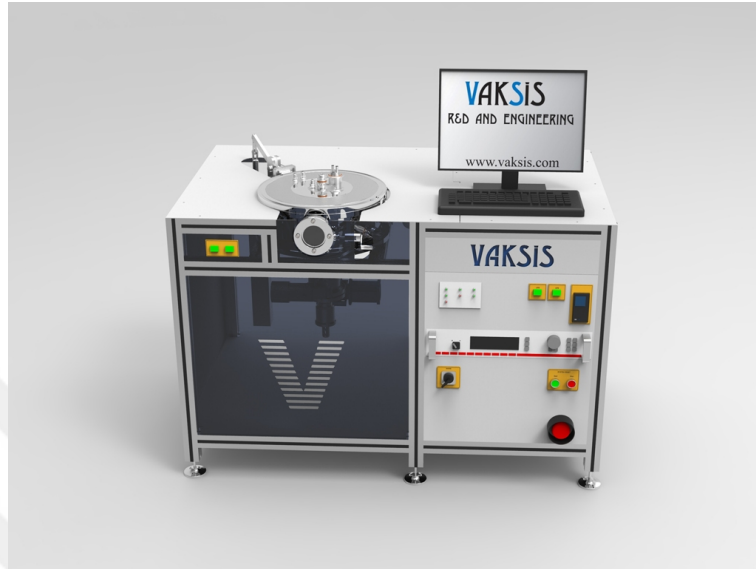
Figure 2.1: Vaksis Handy CVD/PECVD system [39]
