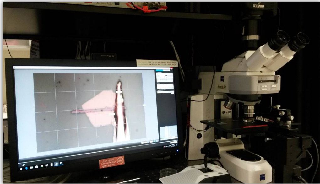
Figure 3.8: A live view that is directly streamed from the camera connected to the microscope to a computer monitor
