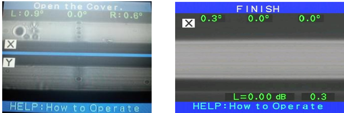
Fig. 6.2.4. The best splice we have obtained in comparison with a perfect splice. The small bubbles in the splice region are the sites for scattering.
